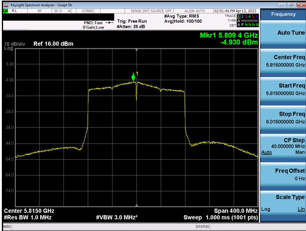
Plot 7-163. Power Spectral Density Plot MIMO ANT2 (160MHz BW 802.11ax (UNII Band 3/4) – Ch. 163)
