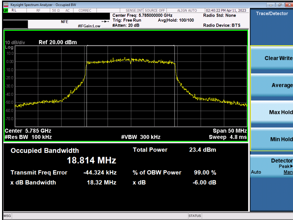
Plot 7-69. 6dB Bandwidth Plot MIMO ANT2 (20MHz BW 802.11ax (UNII Band 3) – Ch. 157)
