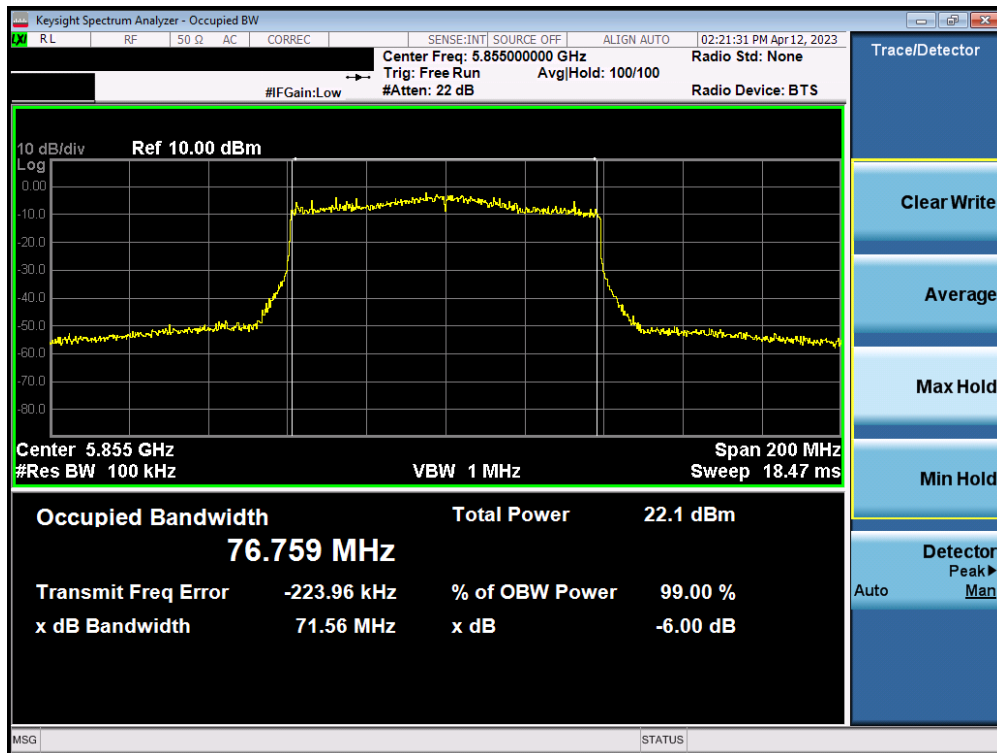
Plot 7-64. 6dB Bandwidth Plot MIMO ANT1 (80MHz BW 802.11ax (UNII Band 3/4) – Ch. 171)
