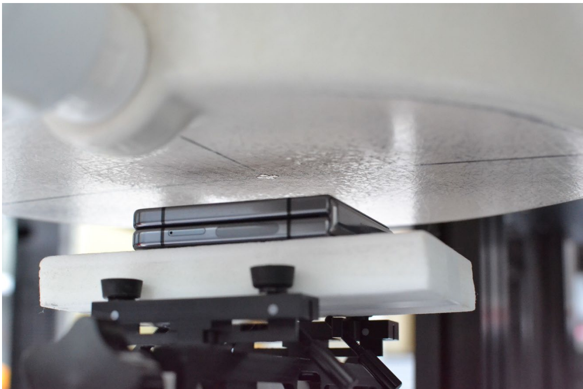
SAR Test Setup Photo 18 – Closed Body-worn, Back Side at 15 mm
