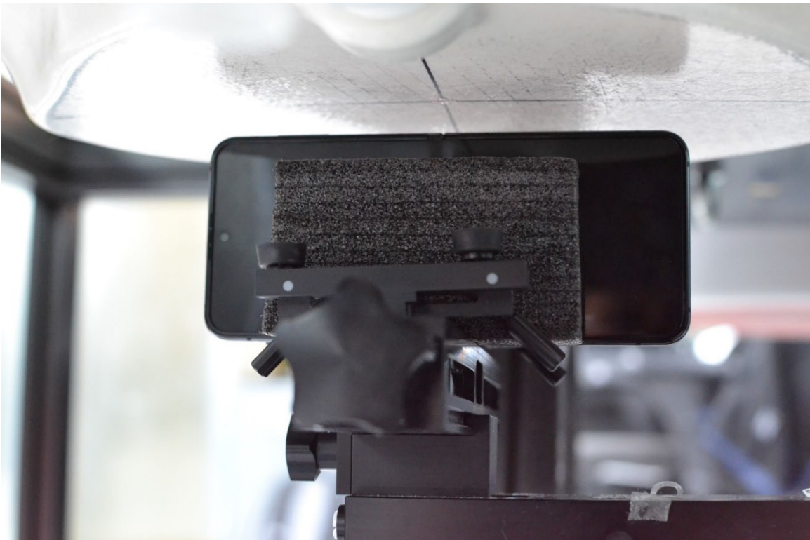
SAR Test Setup Photo 14 – Hotspot, Right Edge at 10 mm
