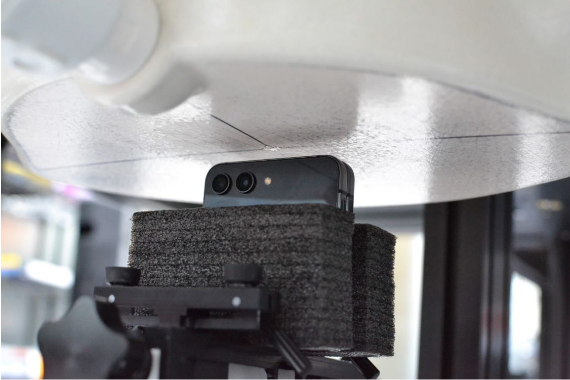
SAR Test Setup Photo 21 – Closed Hotspot, Bottom Edge at 5 mm
