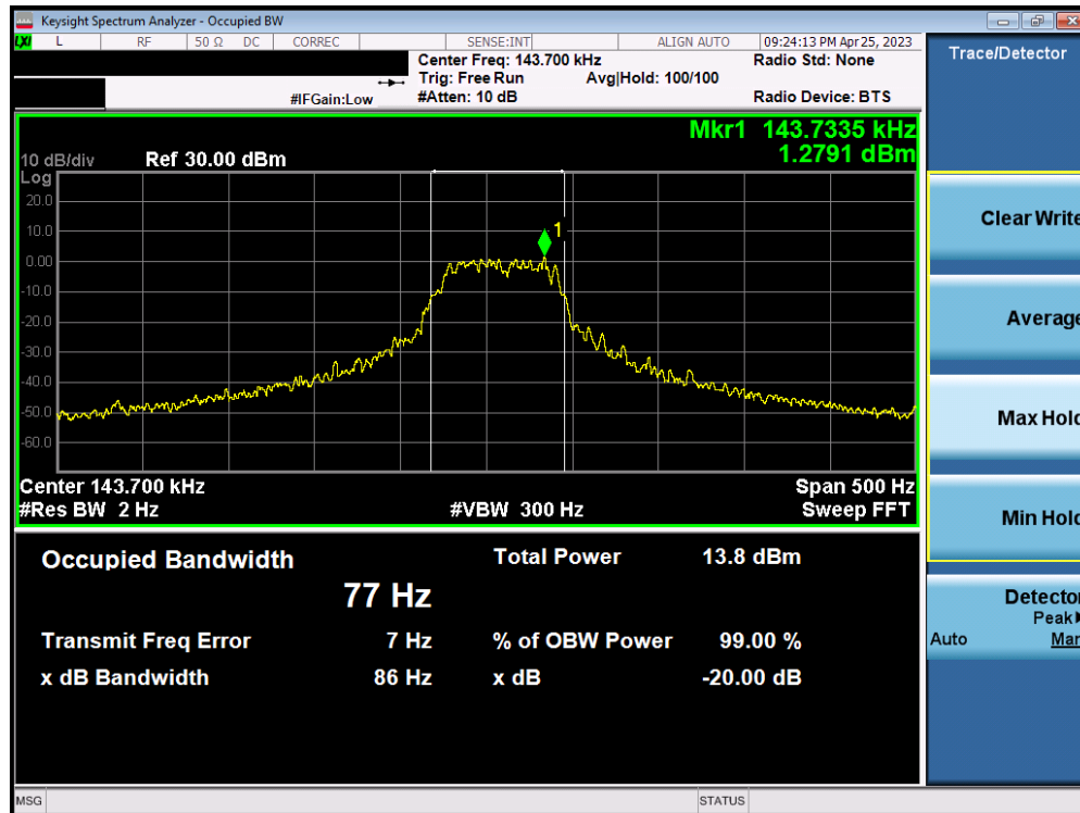
Plot 7-1. Occupied Bandwidth Measurement
