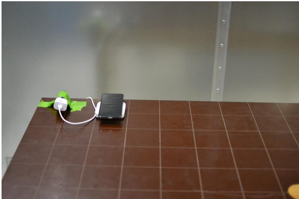
Figure 4. Test Setup – ACLC WCP – <30MHz
