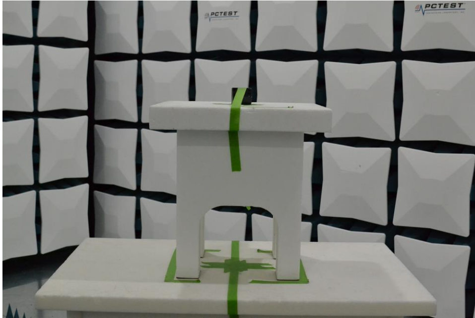
Figure 13. Test Setup – Y Position – 1GHz-18GHz – Closed
