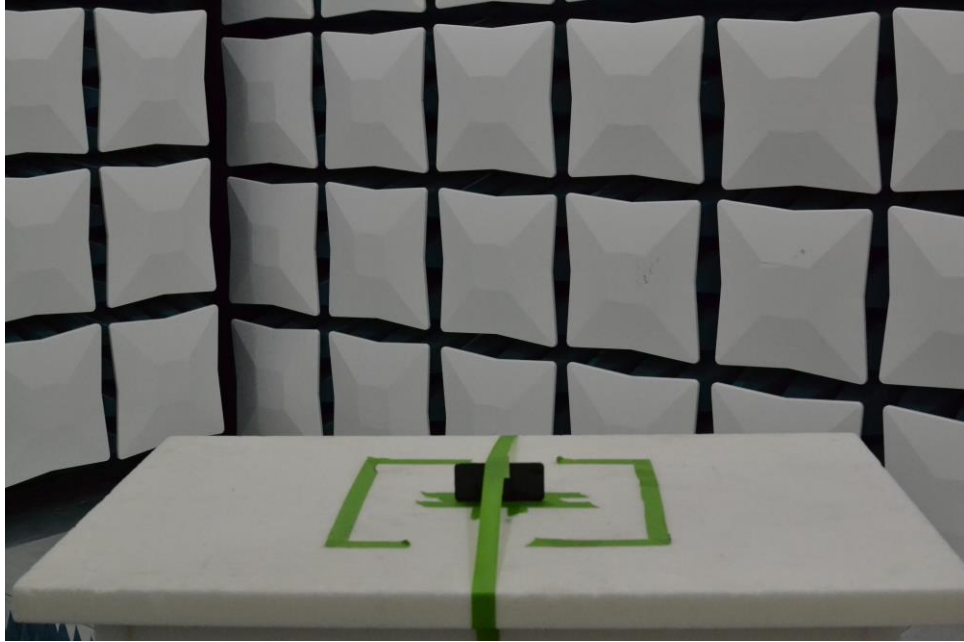
Figure 17. Test Setup – Y Position – 30MHz-1GHz – Open
