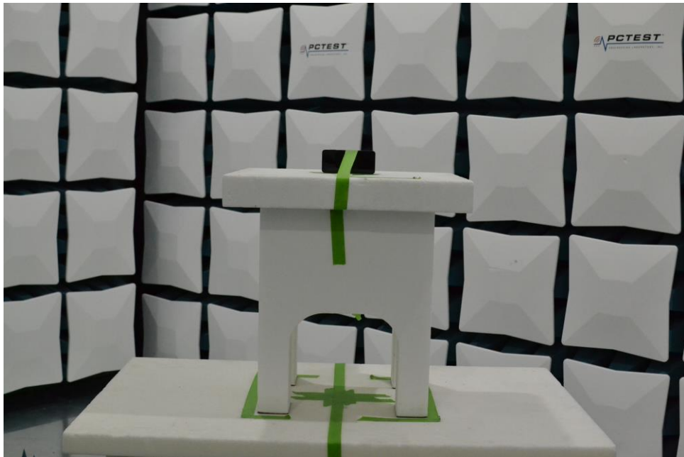
Figure 6. Test Setup – Y Position – 1GHz-18GHz – Open
