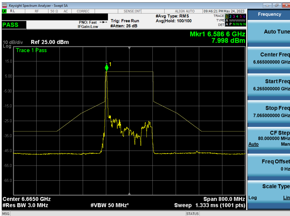
Plot 7-140. In-Band Emission Plot MIMO ANT1 (160MHz BW 802.11ax (26 Tones) (UNII Band 7) – Ch. 143)
