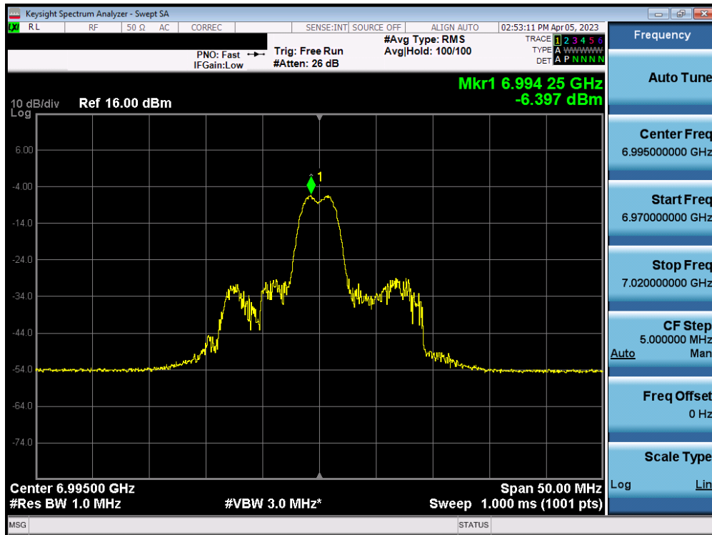
Plot 7-109. Power Spectral Density Plot MIMO ANT2 (20MHz BW 802.11ax (26 Tones) (UNII Band 8) – Ch. 209)
