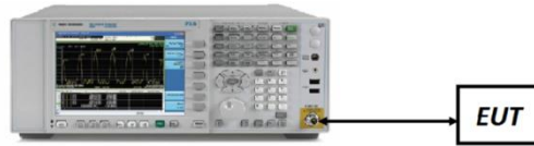
Figure 7-4. Test Instrument & Measurement Setup
