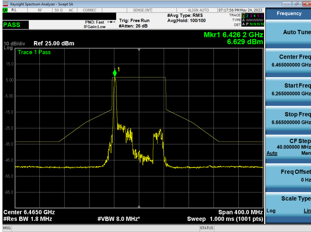
Plot 7-135. In-Band Emission Plot MIMO ANT1 (80MHz BW 802.11ax (26 Tones) (UNII Band 6) – Ch. 103)
