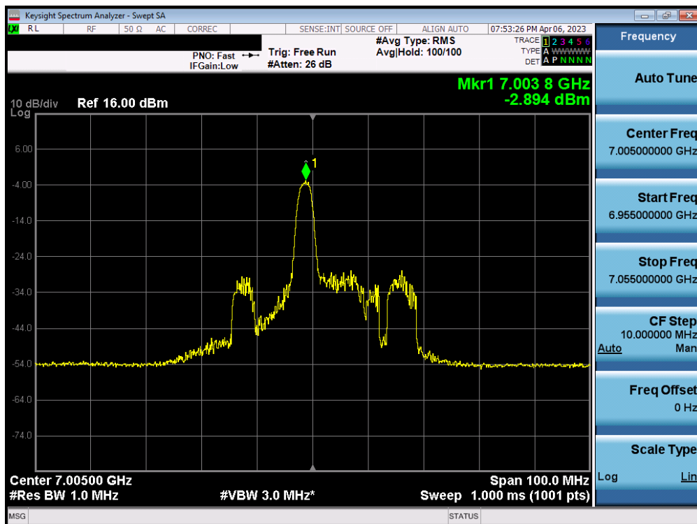
Plot 7-110. Power Spectral Density Plot MIMO ANT2 (40MHz BW 802.11ax (26 Tones) (UNII Band 8) – Ch. 211)
