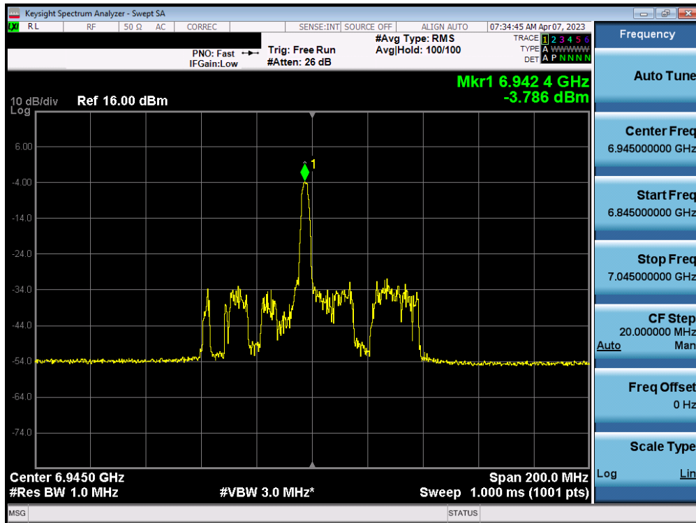
Plot 7-111. Power Spectral Density Plot MIMO ANT2 (80MHz BW 802.11ax (26 Tones) (UNII Band 8) – Ch. 199)
