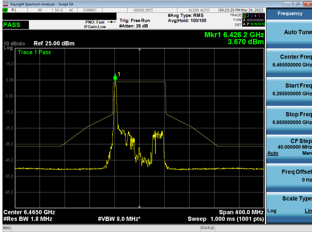
Plot 7-167. In-Band Emission Plot MIMO ANT2 (80MHz BW 802.11ax (26 Tones) (UNII Band 6) – Ch. 103)
