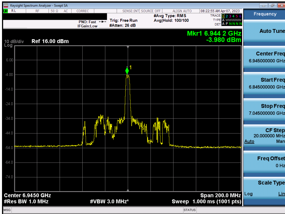
Plot 7-79. Power Spectral Density Plot MIMO ANT1 (80MHz BW 802.11ax (26 Tones) (UNII Band 8) – Ch. 199)
