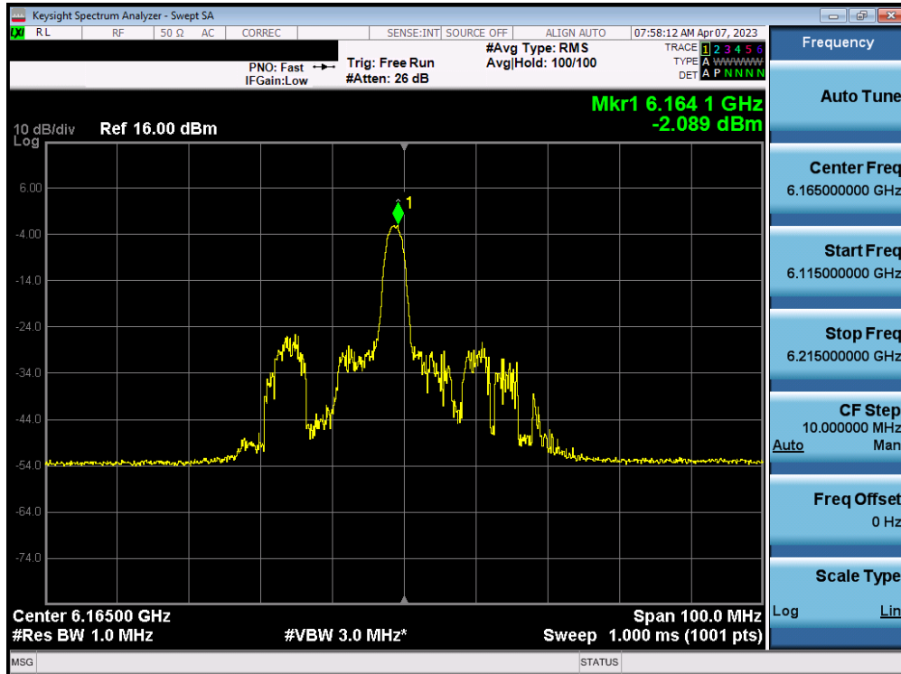
Plot 7-66. Power Spectral Density Plot MIMO ANT1 (40MHz BW 802.11ax (26 Tones) (UNII Band 5) – Ch. 43)
