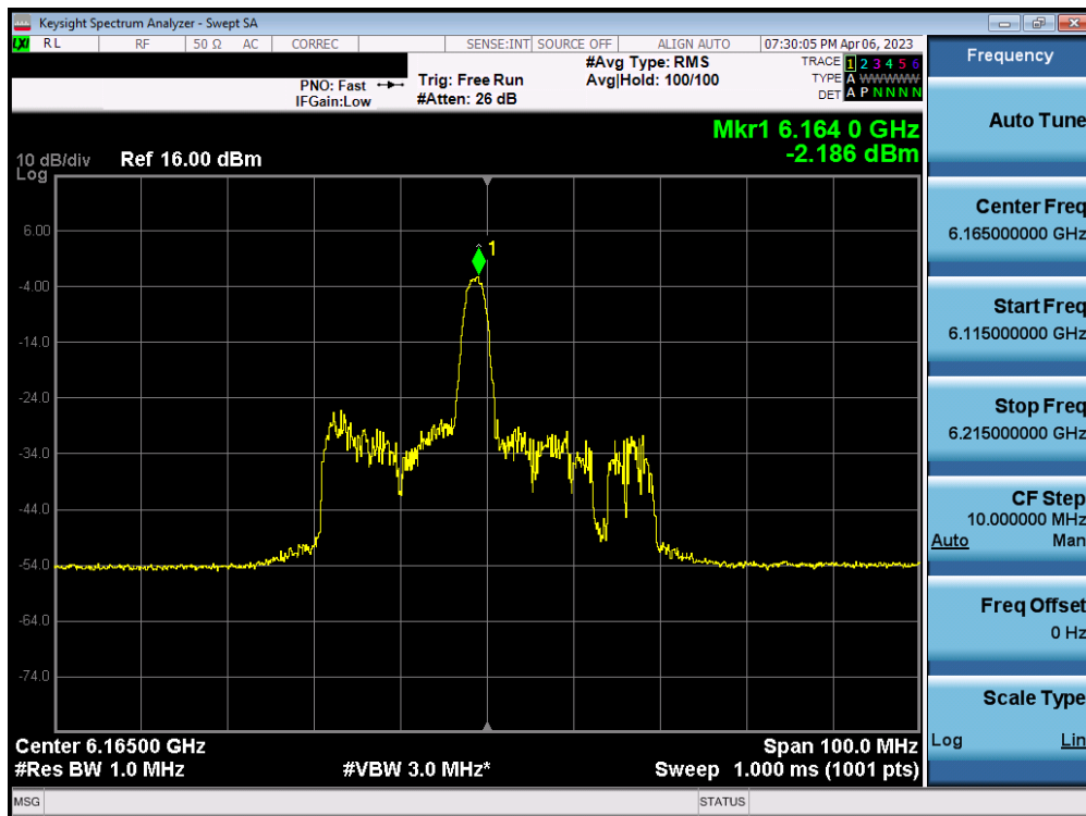
Plot 7-98. Power Spectral Density Plot MIMO ANT2 (40MHz BW 802.11ax (26 Tones) (UNII Band 5) – Ch. 43)
