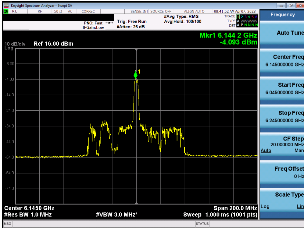
Plot 7-99. Power Spectral Density Plot MIMO ANT2 (80MHz BW 802.11ax (26 Tones) (UNII Band 5) – Ch. 39)
