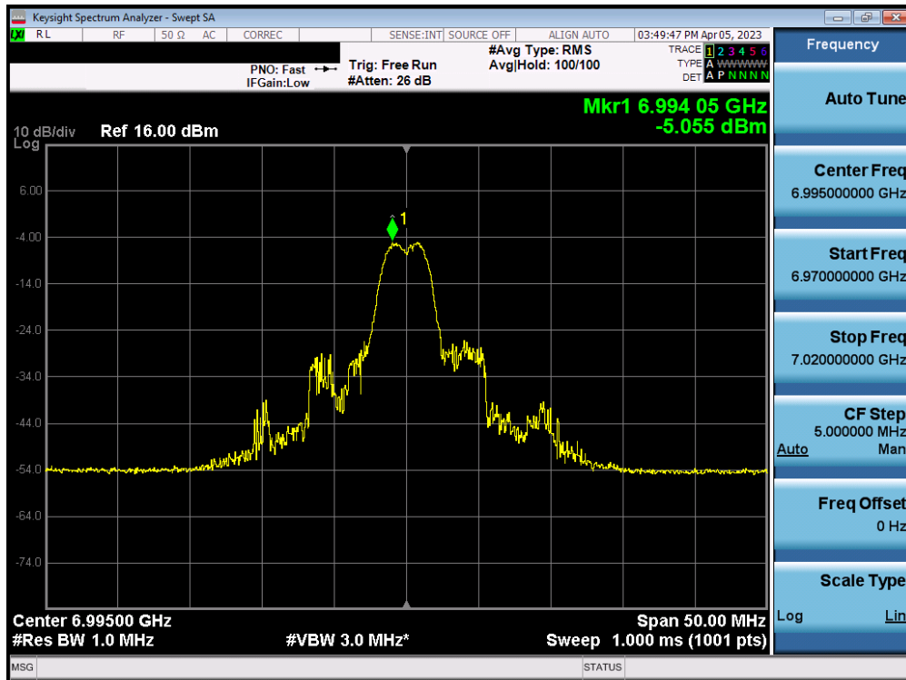
Plot 7-77. Power Spectral Density Plot MIMO ANT1 (20MHz BW 802.11ax (26 Tones) (UNII Band 8) – Ch. 209)
