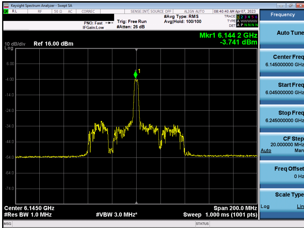
Plot 7-67. Power Spectral Density Plot MIMO ANT1 (80MHz BW 802.11ax (26 Tones) (UNII Band 5) – Ch. 39)
