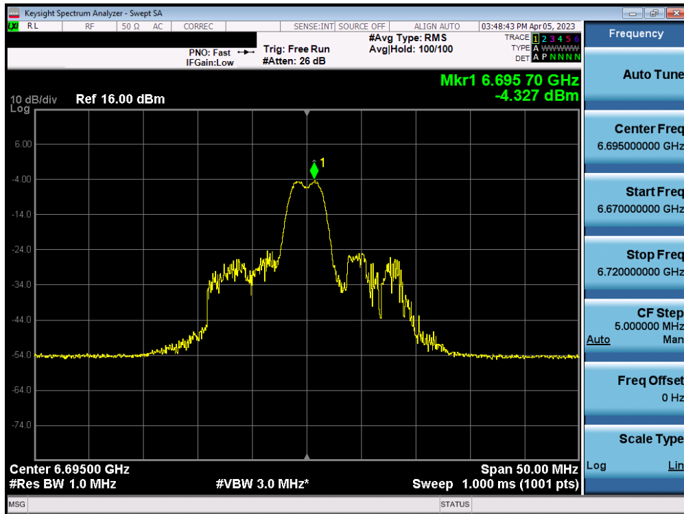
Plot 7-73. Power Spectral Density Plot MIMO ANT1 (20MHz BW 802.11ax (26 Tones) (UNII Band 7) – Ch. 149)
