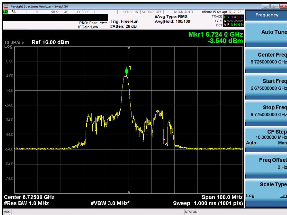
Plot 7-74. Power Spectral Density Plot MIMO ANT1 (40MHz BW 802.11ax (26 Tones) (UNII Band 7) – Ch. 155)
