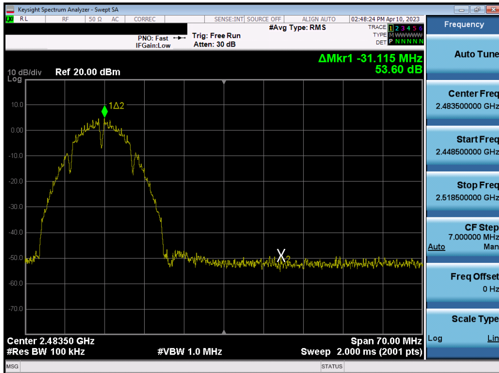
Plot 7-68. Band Edge Plot SISO ANT2 (802.11b – Ch. 11)
