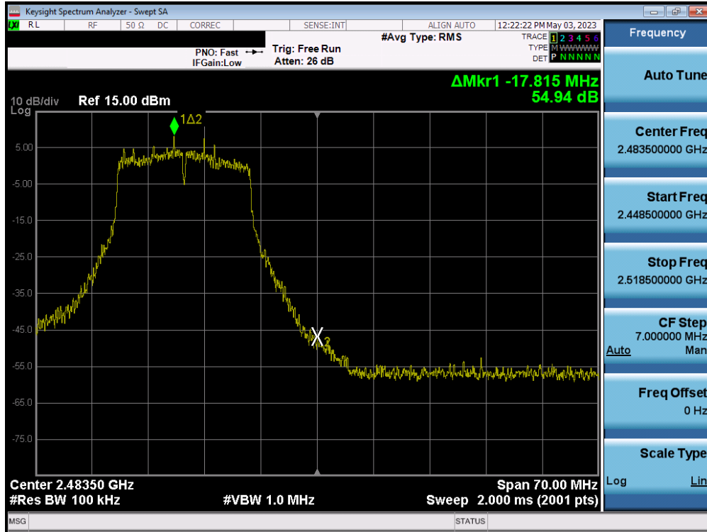
Plot 7-77. Band Edge Plot MIMO ANT1 (802.11g – Ch. 12)
