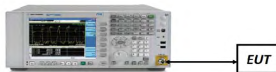
Figure 7-5. Test Instrument & Measurement Setup
