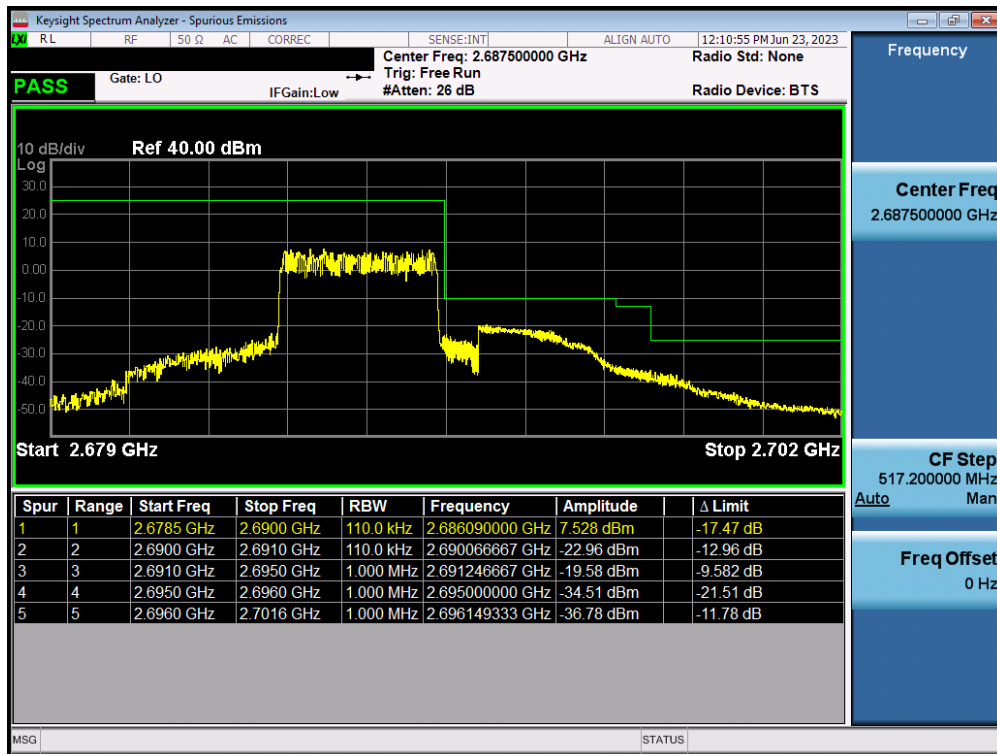
Plot 7-70. Upper ACP Plot (LTE Band 41(PC3) - 5MHz QPSK – Full RB – Ant I)
