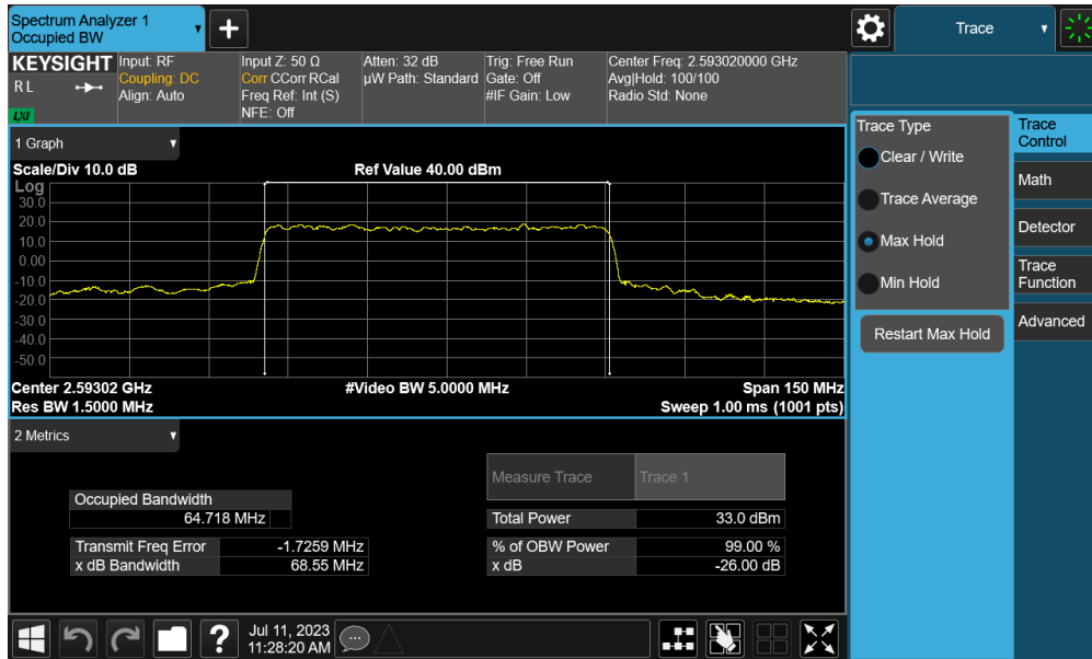
Plot 7-26. Occupied Bandwidth Plot (NR Band n41 - 70MHz π/2 BPSK - Full RB – Ant I)
