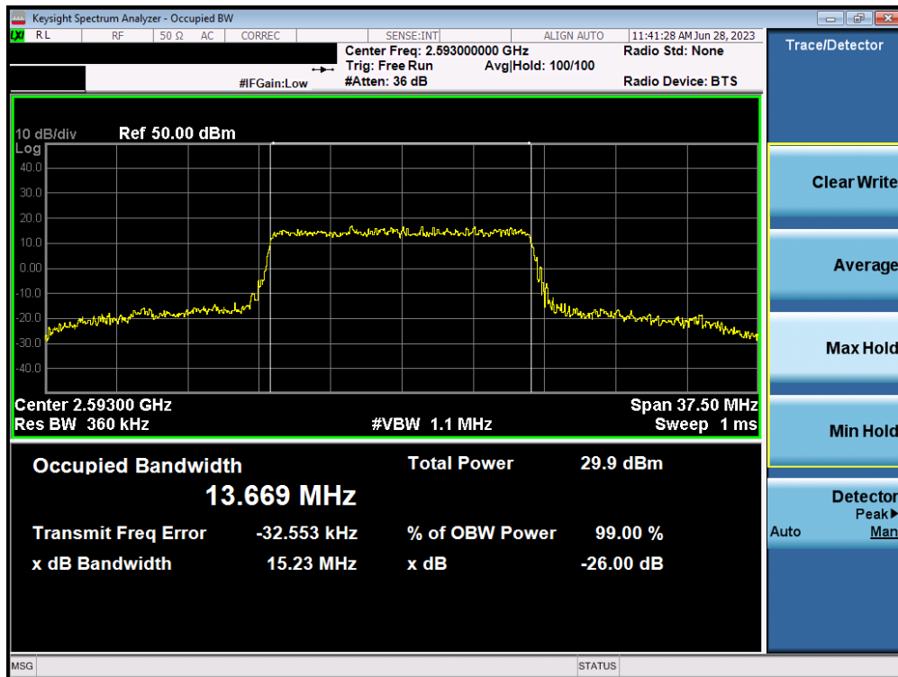
Plot 7-46. Occupied Bandwidth Plot (NR Band n41 - 15MHz 16-QAM - Full RB - Ant I)
