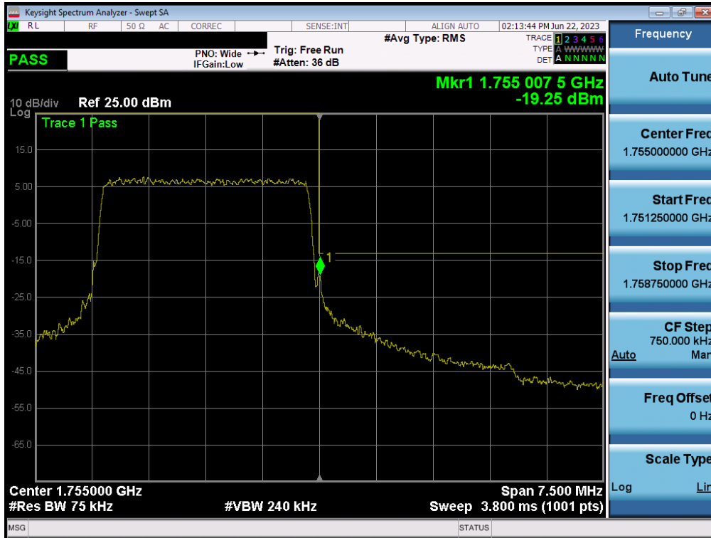
Plot 7-101. Upper Band Edge Plot (LTE Band 4 - 3MHz QPSK – Full RB – Ant A)
