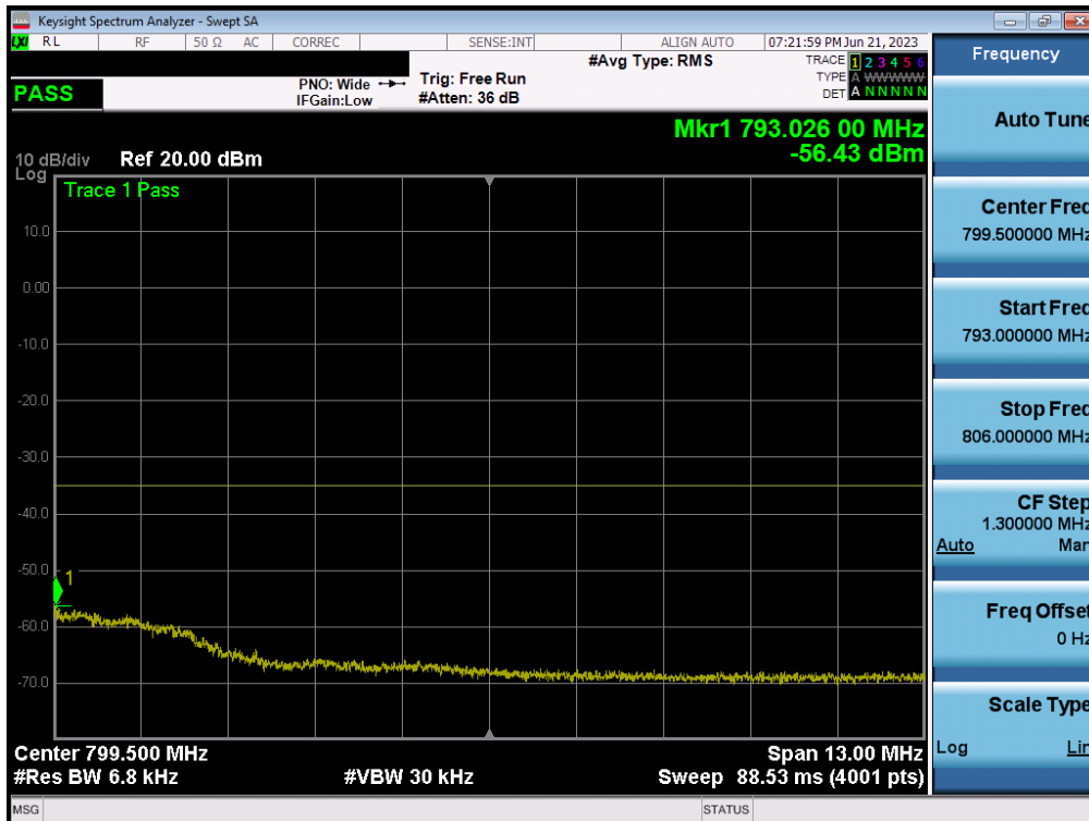
Plot 7-98. Upper Emission Mask Plot (LTE Band 13 - 5MHz QPSK – Full RB – Ant A)
