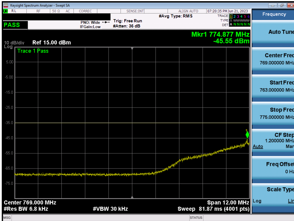
Plot 7-96. Lower Emission Mask Plot (LTE Band 13 - 5MHz QPSK – Full RB – Ant A)
