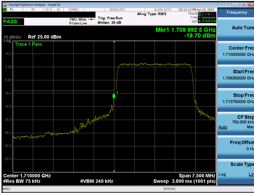
Plot 7-99. Lower Band Edge Plot (LTE Band 66/4 - 3MHz QPSK – Full RB – Ant A)
