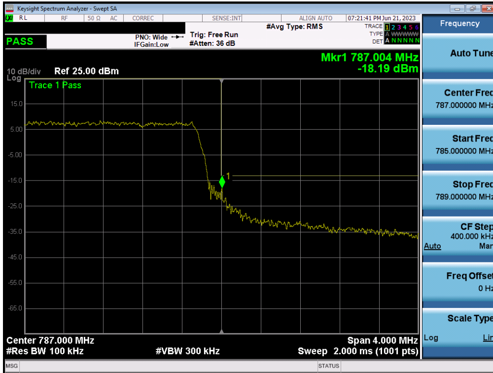
Plot 7-97. Upper Band Edge Plot (LTE Band 13 - 5MHz QPSK – Full RB – Ant A)
