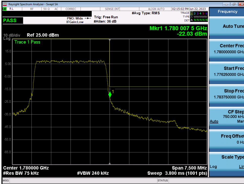
Plot 7-103. Upper Band Edge Plot (LTE Band 66 - 3MHz QPSK – Full RB – Ant A)
