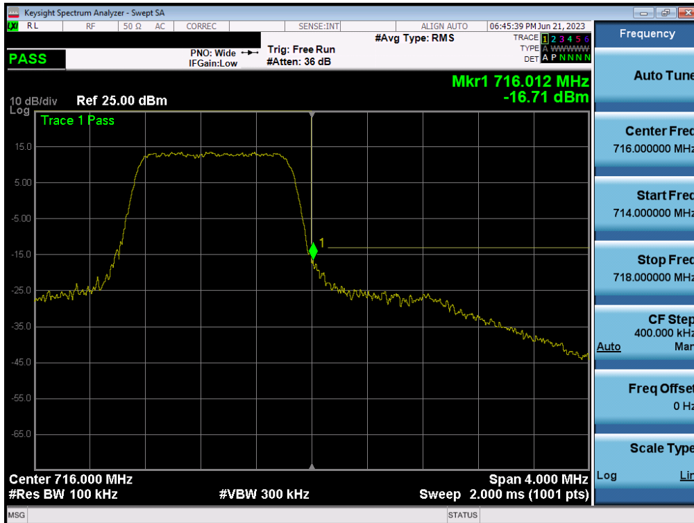
Plot 7-94. Upper Band Edge Plot (LTE Band 12 – 1.4MHz QPSK – Full RB – Ant A)
