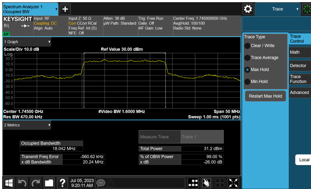
Plot 7-63. Occupied Bandwidth Plot (NR Band n66 - 20.0MHz DFT-s-OFDM BPSK - Full RB – Ant I)
