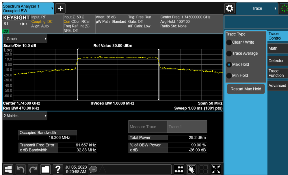
Plot 7-65. Occupied Bandwidth Plot (NR Band n66 - 20.0MHz CP-OFDM 16QAM - Full RB - Ant I)
