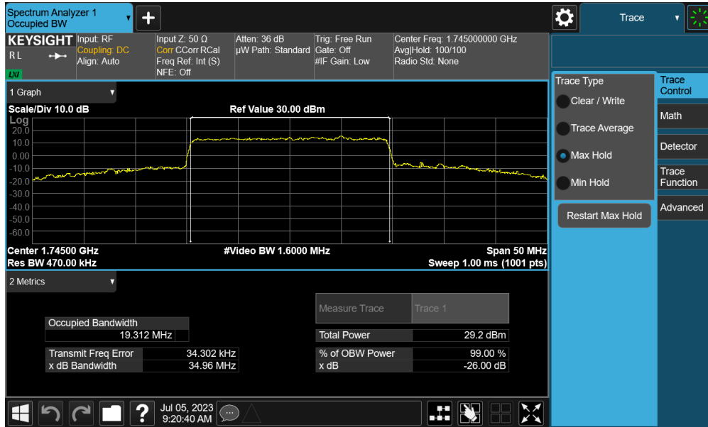
Plot 7-64. Occupied Bandwidth Plot (NR Band n66 - 20.0MHz CP-OFDM QPSK - Full RB - Ant I)
