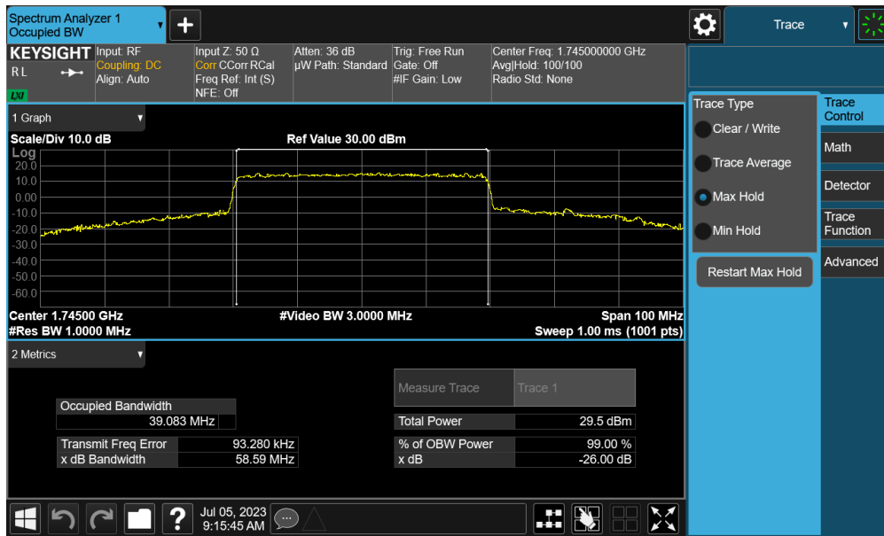
Plot 7-55. Occupied Bandwidth Plot (NR Band n66 - 40.0MHz CP-OFDM QPSK - Full RB – Ant I)
