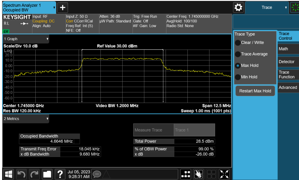
Plot 7-74. Occupied Bandwidth Plot (NR Band n66 - 5.0MHz CP-OFDM 16QAM - Full RB – Ant I)
