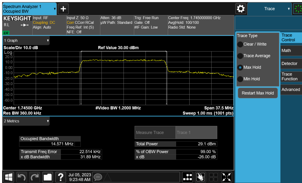
Plot 7-67. Occupied Bandwidth Plot (NR Band n66 - 15.0MHz CP-OFDM QPSK - Full RB - Ant I)
