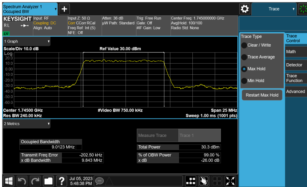
Plot 7-36. Occupied Bandwidth Plot (NR Band n66 - 10.0MHz DFT-s-OFDM BPSK - Full RB - Ant A)
