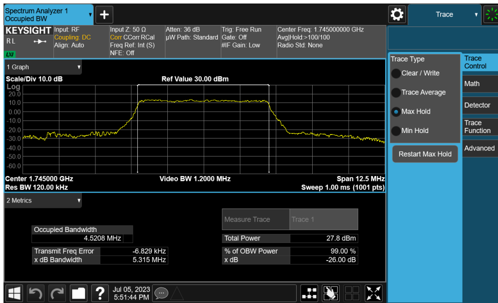
Plot 7-40. Occupied Bandwidth Plot (NR Band n66 - 5.0MHz CP-OFDM QPSK - Full RB - Ant A)
