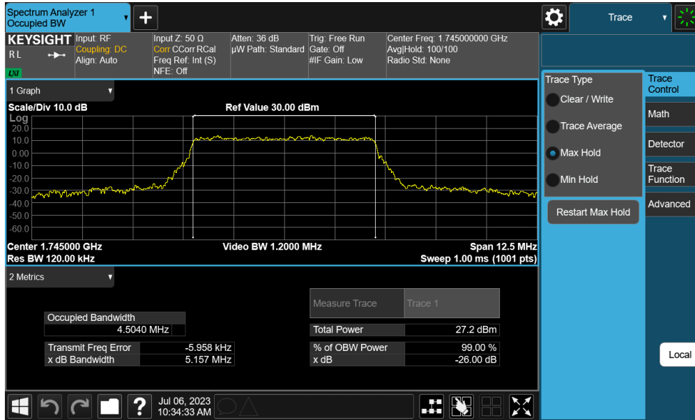
Plot 7-41. Occupied Bandwidth Plot (NR Band n66 - 5.0MHz CP-OFDM 16QAM - Full RB – Ant A)
