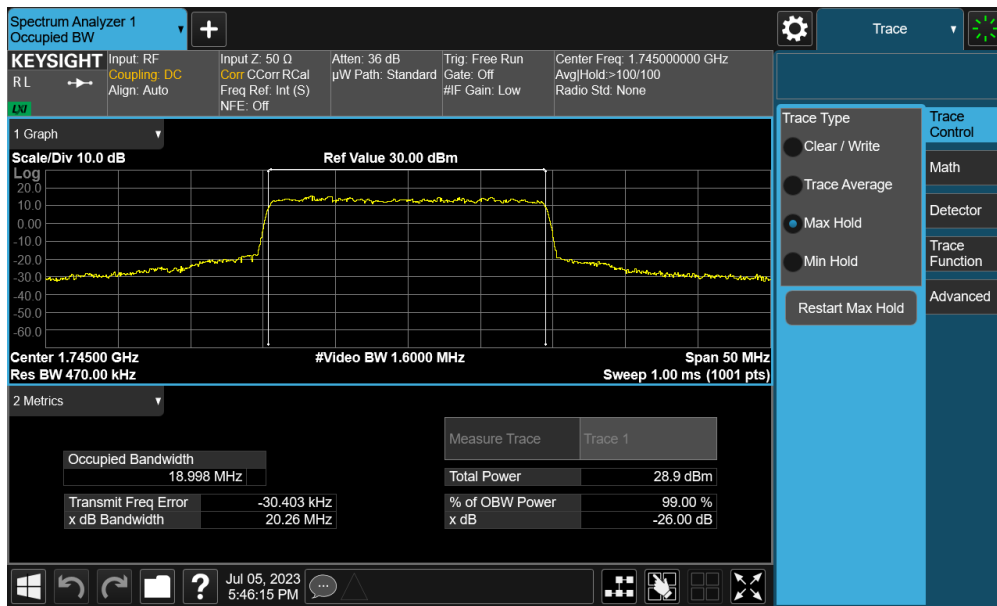
Plot 7-32. Occupied Bandwidth Plot (NR Band n66 - 20.0MHz CP-OFDM 16QAM - Full RB – Ant A)
