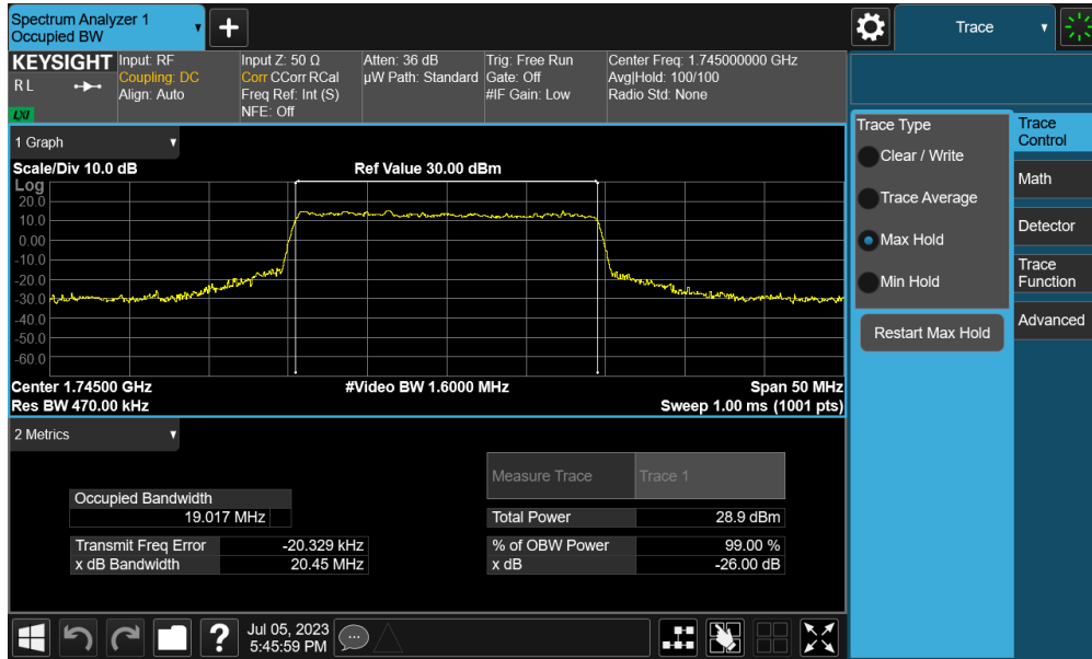
Plot 7-31. Occupied Bandwidth Plot (NR Band n66 - 20.0MHz CP-OFDM QPSK - Full RB – Ant A)
