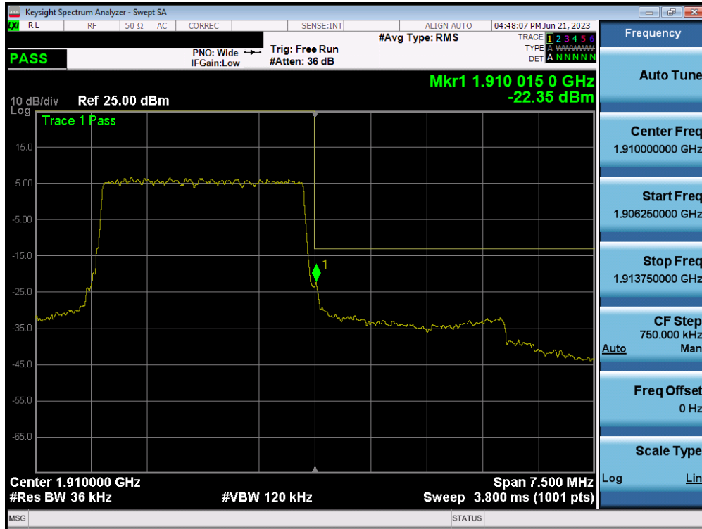
Plot 7-44. Upper Band Edge Plot (LTE Band 2 - 3MHz QPSK – Full RB – Ant I)
