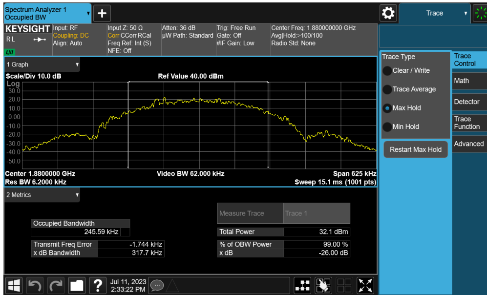
Plot 7-14. Occupied Bandwidth Plot (EDGE, Ch. 661 – Ant A)
