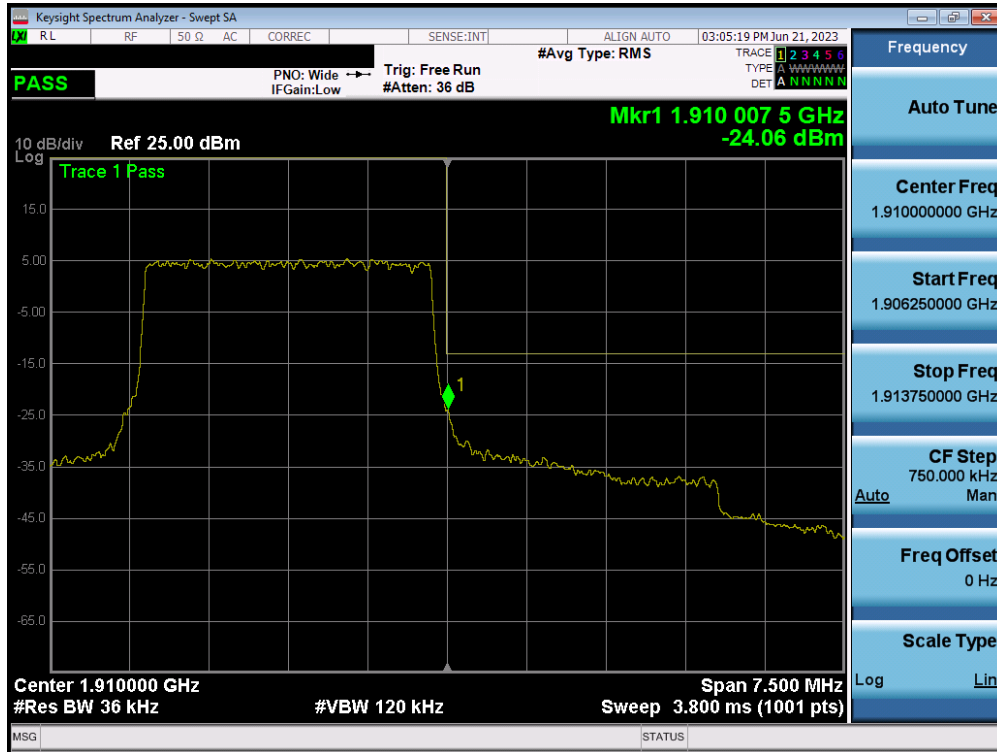
Plot 7-38. Upper Band Edge Plot (LTE Band 2 - 3MHz QPSK – Full RB – Ant A)
