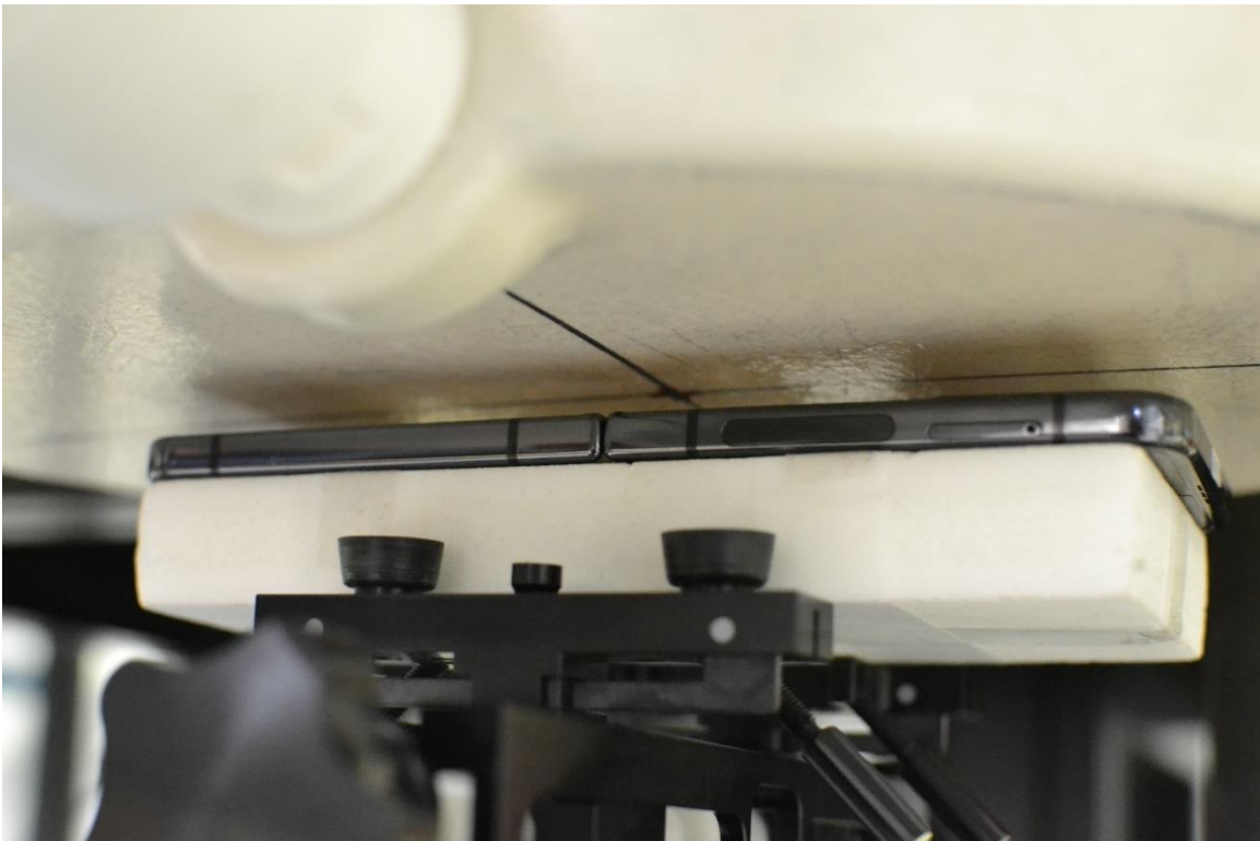
SAR Test Setup Photo 6 – Hotspot, Back Side at 10 mm
