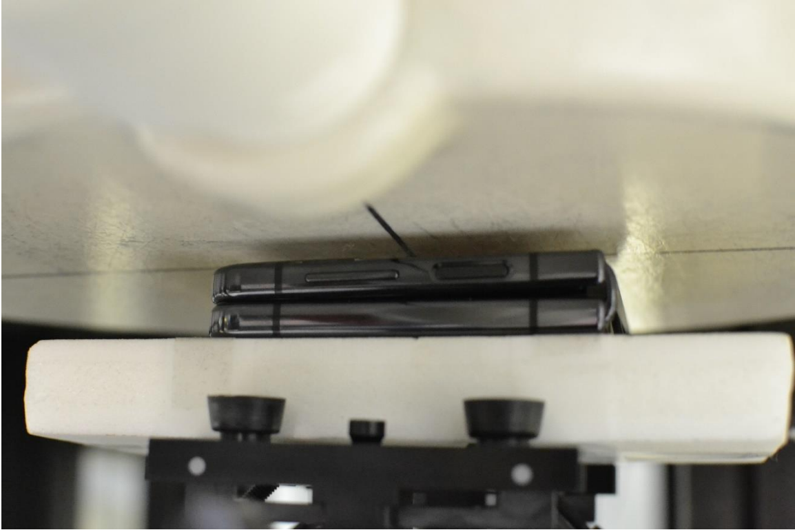
SAR Test Setup Photo 23 – Closed Hotspot, Front Side at 5 mm
