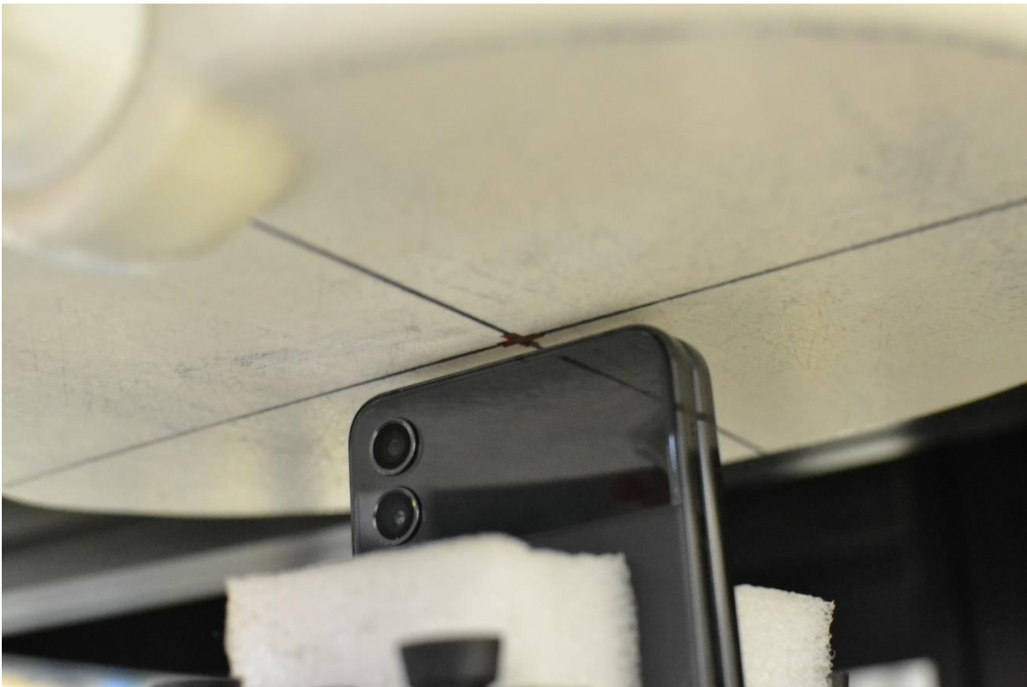
SAR Test Setup Photo 24 – Closed Hotspot, Bottom Edge at 5 mm
