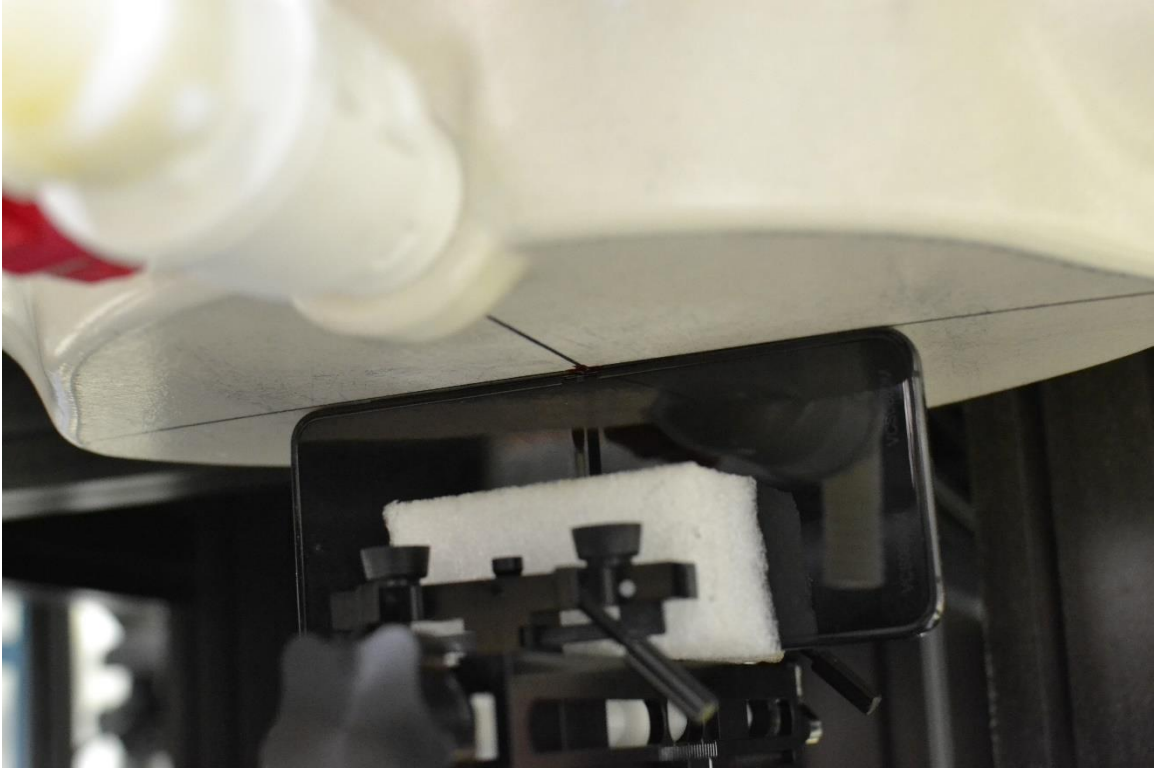
SAR Test Setup Photo 17 – Phablet, Right Edge at 0 mm
