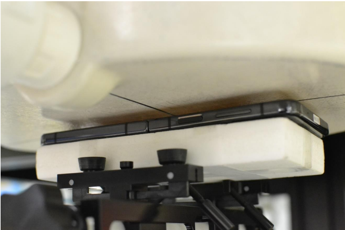
SAR Test Setup Photo 10 – Phablet, Front Side at 6 mm
