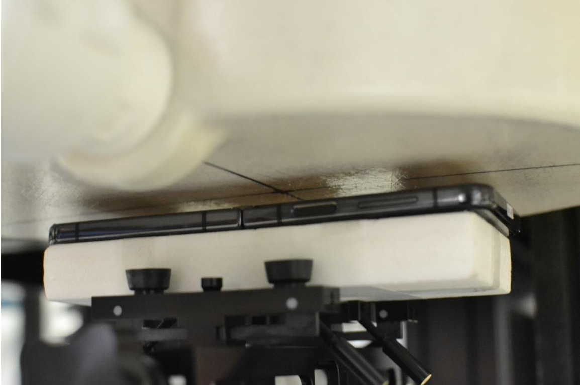
SAR Test Setup Photo 9 – Hotspot, Front Side at 10 mm
