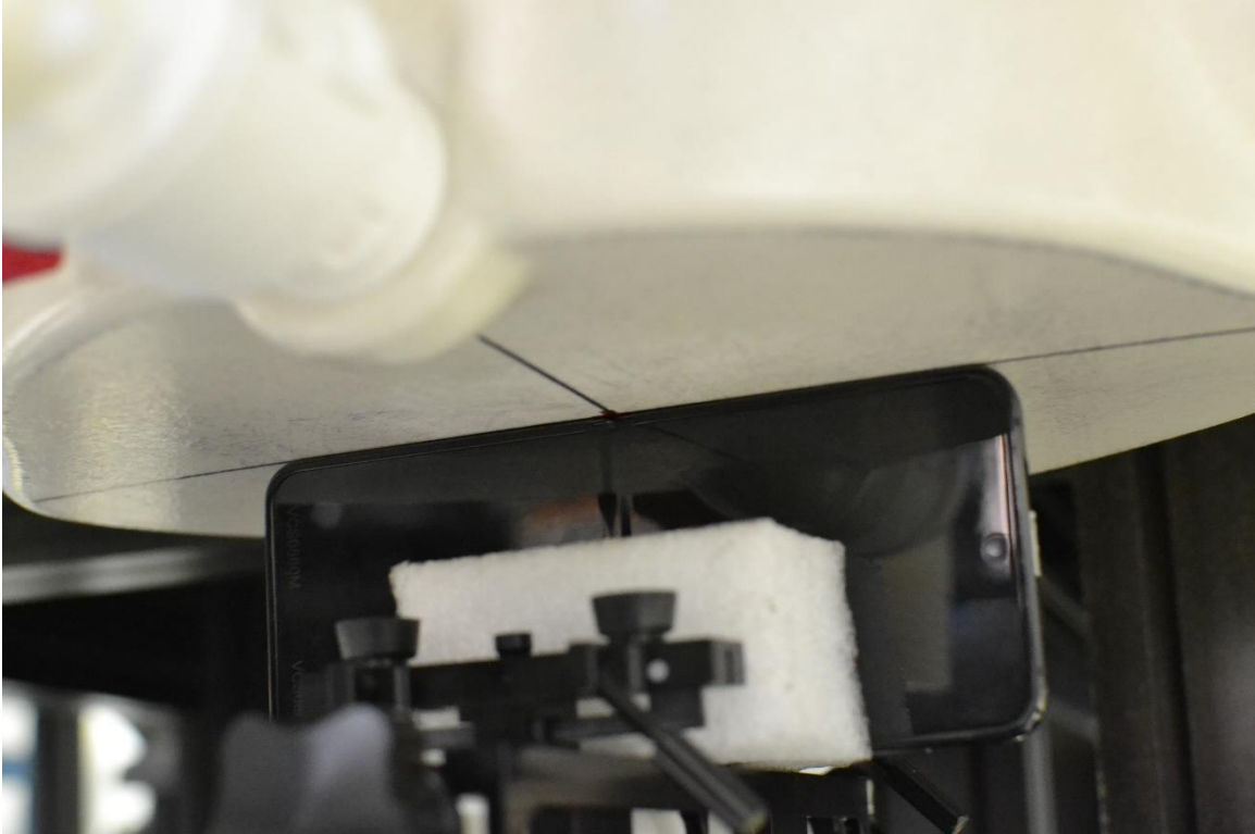
SAR Test Setup Photo 19 – Phablet, Left Edge at 0 mm
