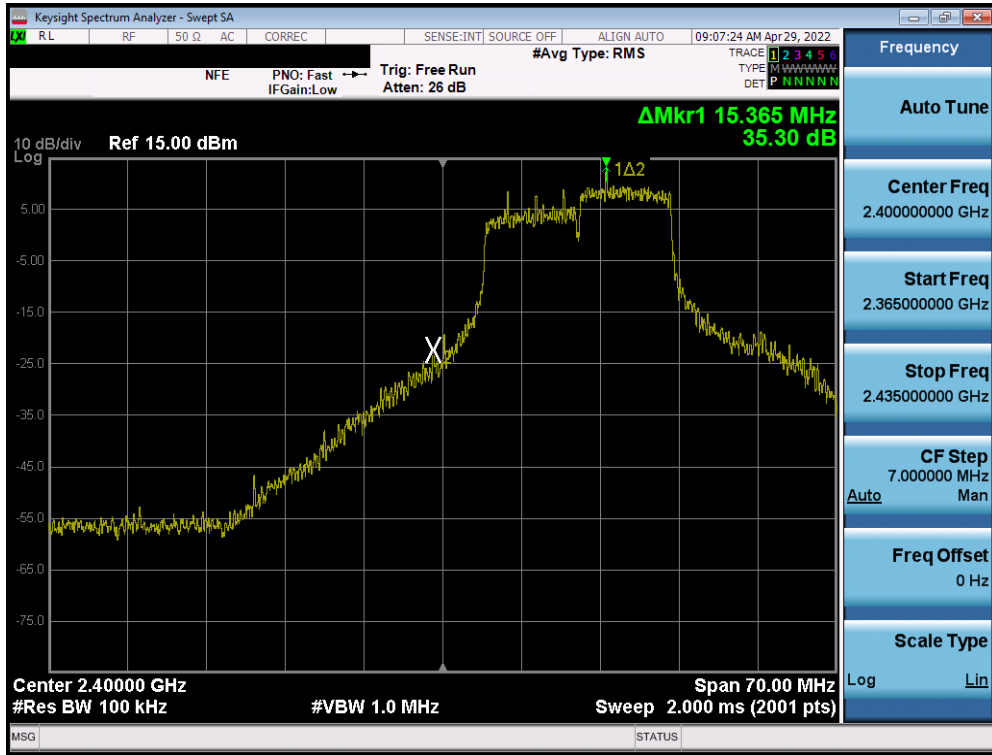
Plot 7-59. Band Edge Plot SISO ANT2 (802.11g- Ch. 1)
