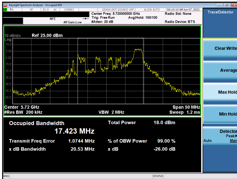
Plot 7-67. 26dB Bandwidth Plot ANT2 (20MHz BW 802.11ax – 26 Tones (UNII Band 2C) – Ch. 144)
