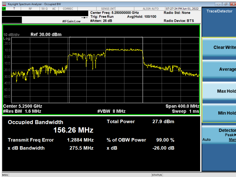
Plot 7-33. 26dB Bandwidth Plot SISO ANT1 (160MHz U BW 802.11ax – 996 Tones (UNII Band 1/2A) – Ch. 50)
