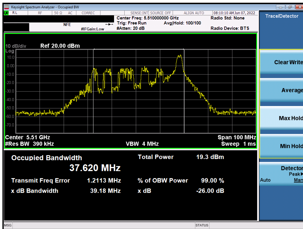
Plot 7-18. 26dB Bandwidth Plot SISO ANT1 (40MHz BW 802.11ax – 26 Tones (UNII Band 2C) – Ch. 102)
