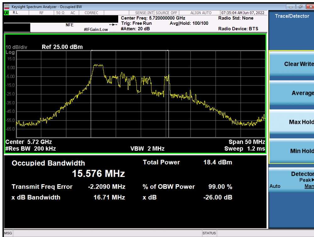
Plot 7-17. 26dB Bandwidth Plot SISO ANT1 (20MHz BW 802.11ax – 26 Tones (UNII Band 2C) – Ch. 144)
