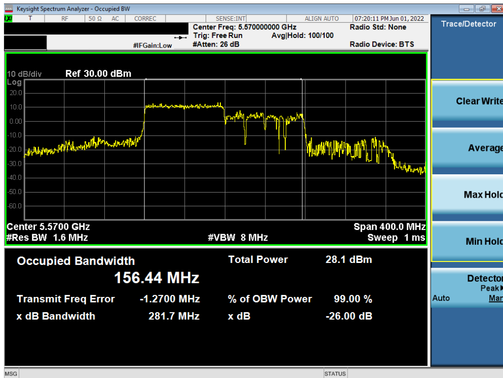
Plot 7-49. 26dB Bandwidth Plot SISO ANT1 (160MHz L BW 802.11ax – 996 Tones (UNII Band 2C) – Ch. 114)
