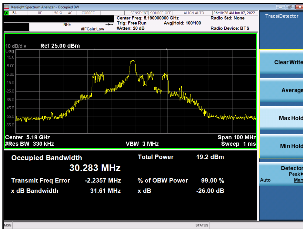
Plot 7-54. 26dB Bandwidth Plot ANT2 (40MHz BW 802.11ax – 26 Tones (UNII Band 1) – Ch. 38)
