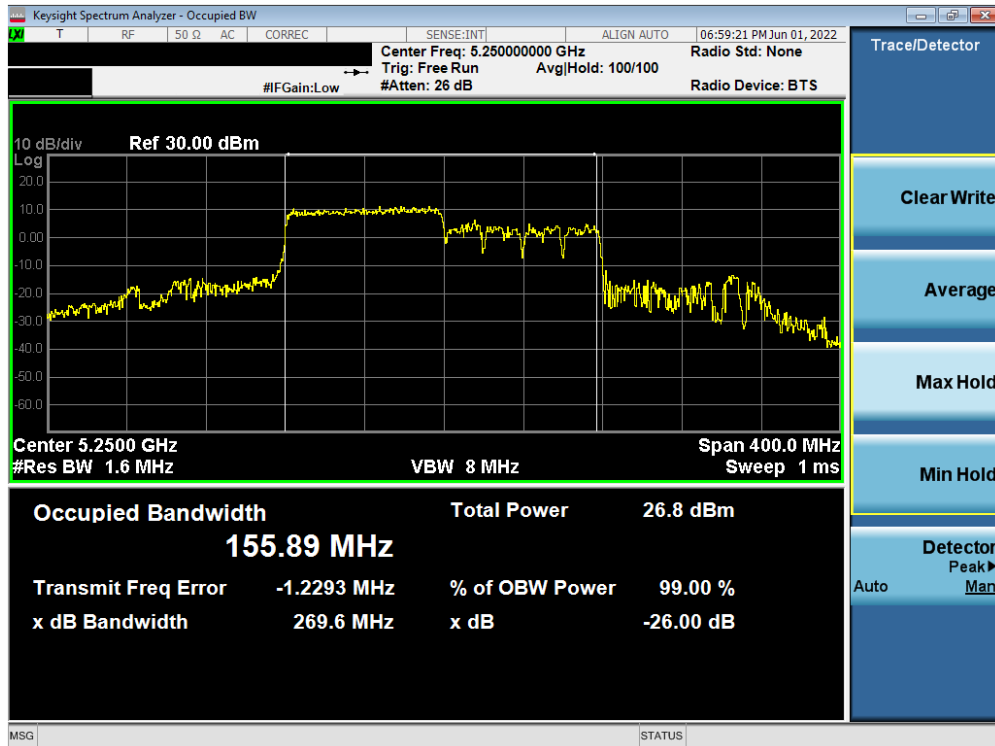
Plot 7-82. 26dB Bandwidth Plot ANT2 (160MHz L BW 802.11ax – 996 Tones (UNII Band 1/2A) – Ch. 50)
