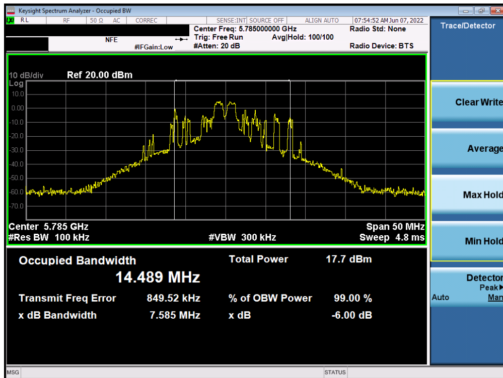
Plot 7-102. 6dB Bandwidth Plot SISO ANT1 (20MHz BW 802.11ax – 26 Tones (UNII Band 3) – Ch. 157)
