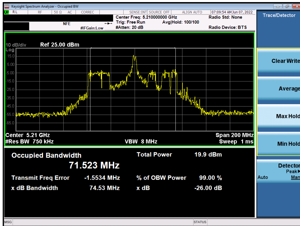
Plot 7-56. 26dB Bandwidth Plot ANT2 (80MHz BW 802.11ax – 26 Tones (UNII Band 1) – Ch. 42)
