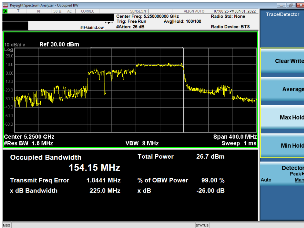
Plot 7-83. 26dB Bandwidth Plot ANT2 (160MHz U BW 802.11ax – 996 Tones (UNII Band 1/2A) – Ch. 50)
