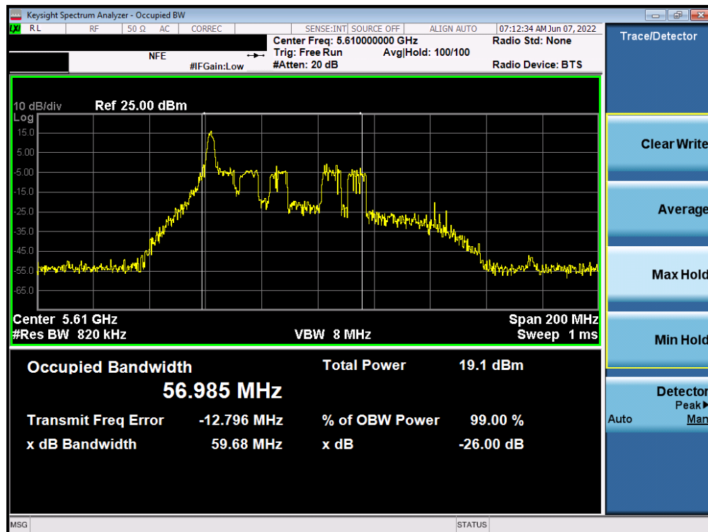
Plot 7-72. 26dB Bandwidth Plot ANT2 (80MHz BW 802.11ax – 26 Tones (UNII Band 2C) – Ch. 122)
