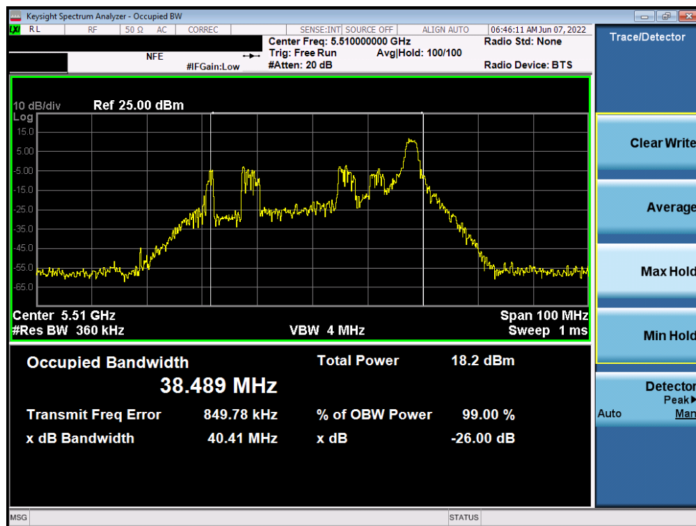
Plot 7-68. 26dB Bandwidth Plot ANT2 (40MHz BW 802.11ax – 26 Tones (UNII Band 2C) – Ch. 102)
