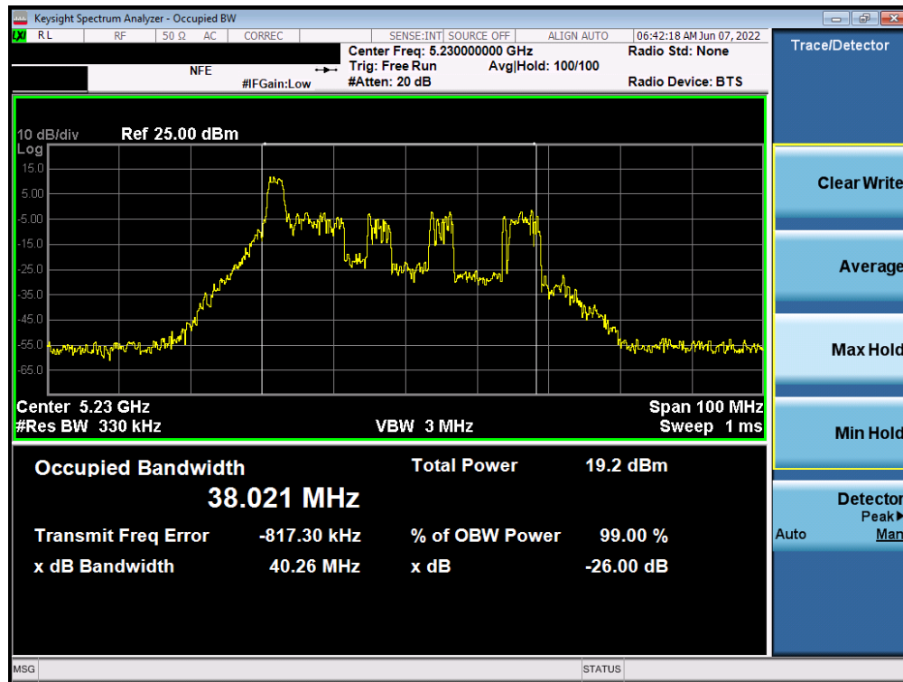
Plot 7-55. 26dB Bandwidth Plot ANT2 (40MHz BW 802.11ax – 26 Tones (UNII Band 1) – Ch. 46)
