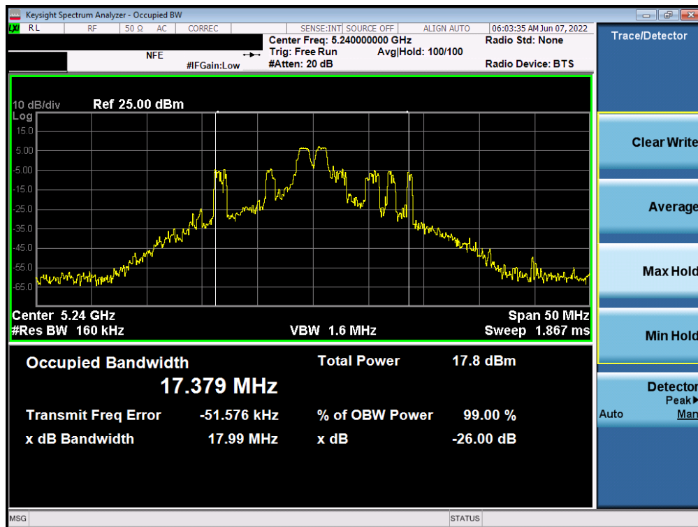
Plot 7-53. 26dB Bandwidth Plot ANT2 (20MHz BW 802.11ax – 26 Tones (UNII Band 1) – Ch. 48)
