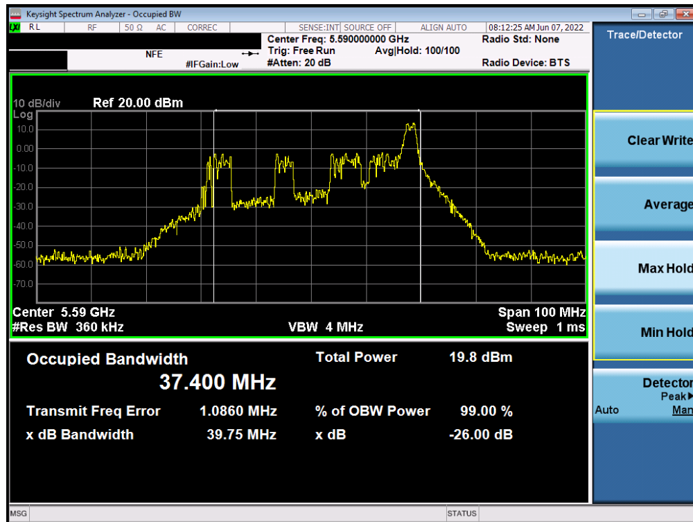
Plot 7-19. 26dB Bandwidth Plot SISO ANT1 (40MHz BW 802.11ax – 26 Tones (UNII Band 2C) – Ch. 118)
