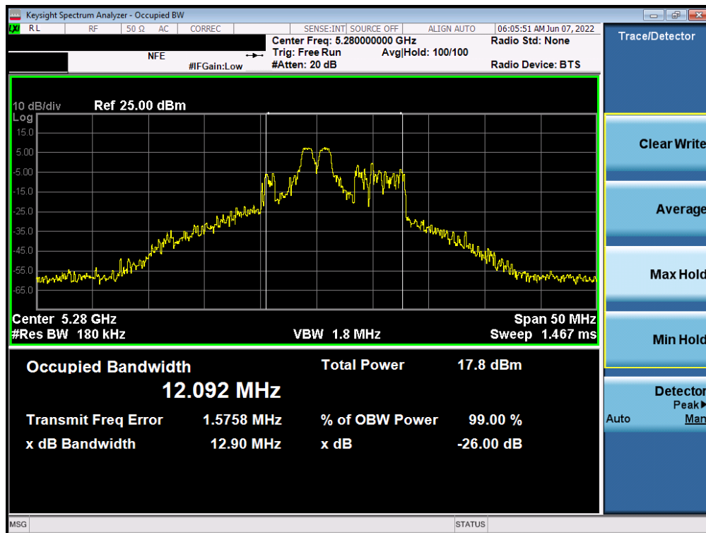
Plot 7-60. 26dB Bandwidth Plot ANT2 (20MHz BW 802.11ax – 26 Tones (UNII Band 2A) – Ch. 56)
