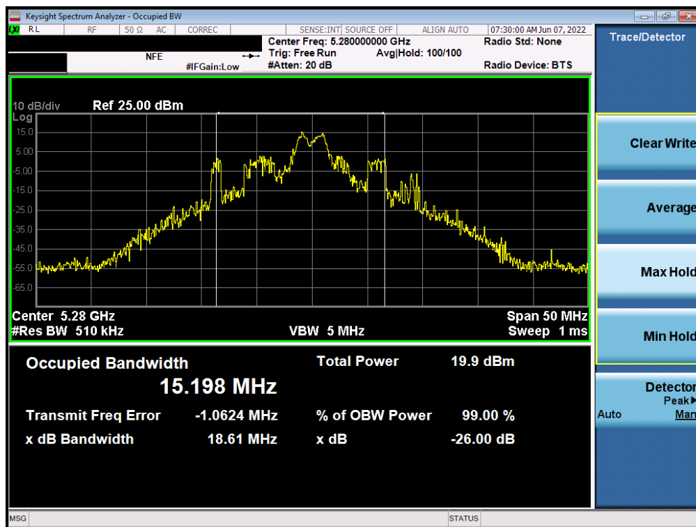
Plot 7-10. 26dB Bandwidth Plot SISO ANT1 (20MHz BW 802.11ax – 26 Tones (UNII Band 2A) – Ch. 56)
