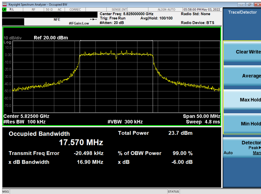
Plot 7-153. 6dB Bandwidth Plot ANT2 (20MHz BW 802.11n (UNII Band 3) – Ch. 165)
