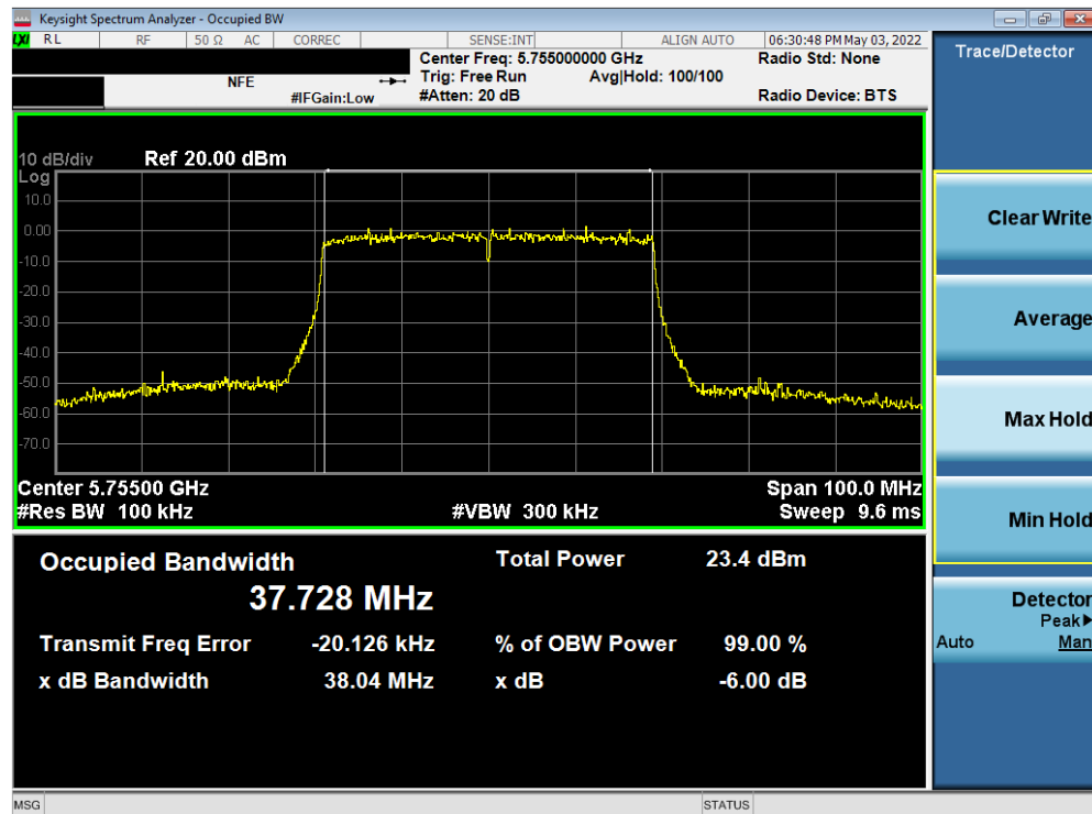
Plot 7-122. 6dB Bandwidth Plot SISO ANT1 (40MHz BW 802.11ax (UNII Band 3) – Ch. 151)
