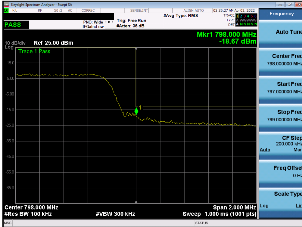
Plot 7-27. Upper Band Edge Plot (LTE Band 14, 5MHz QPSK - RB Size 25)
