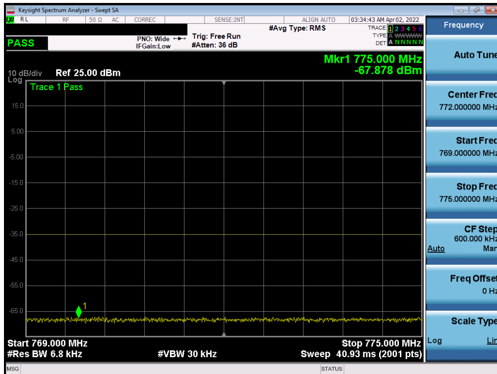
Plot 7-26. Lower Emission Mask Plot (LTE Band 14, 5MHz QPSK - RB Size 25)
