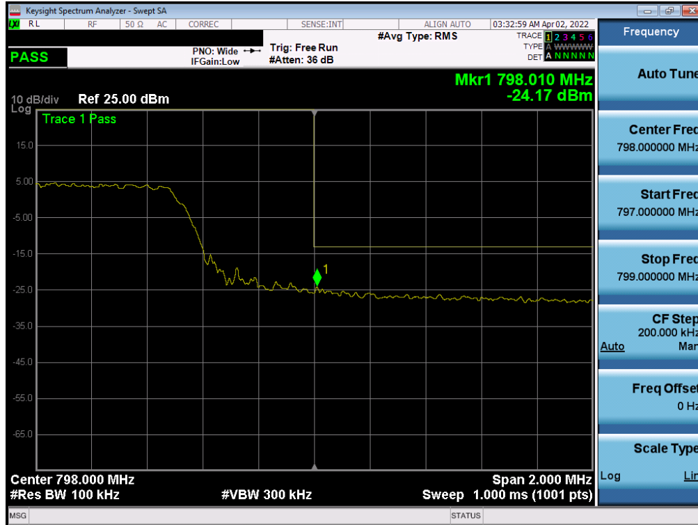
Plot 7-23. Upper Band Edge Plot (LTE Band 14, 10MHz QPSK - RB Size 50)
