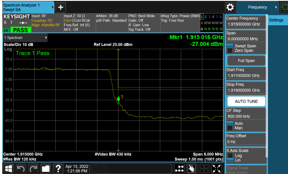
Plot 7-203. Upper Band Edge Plot (NR Band n25 - 10MHz QPSK – Full RB)
