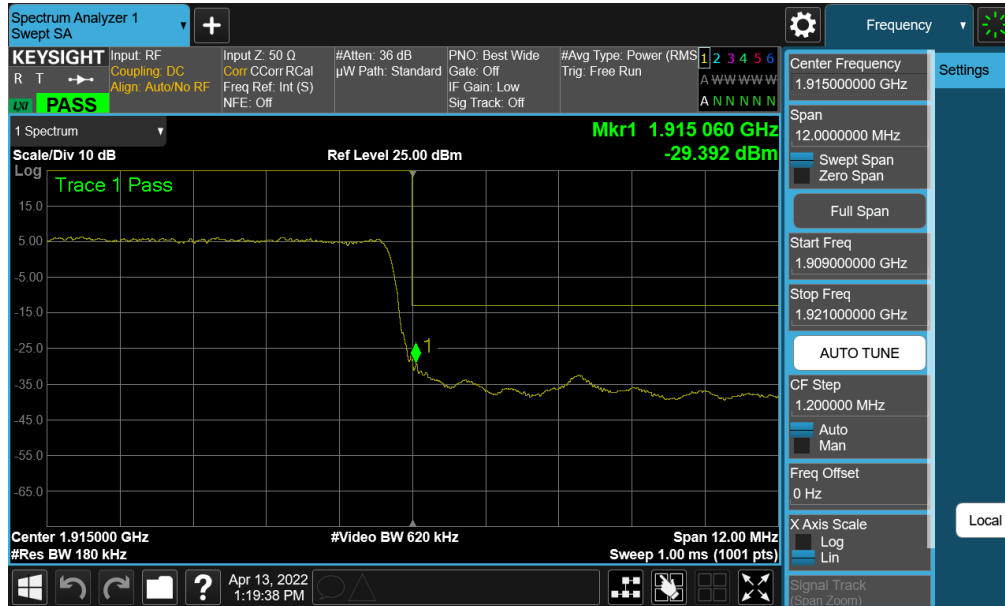
Plot 7-197. Upper Band Edge Plot (NR Band n25 - 15MHz QPSK – Full RB)
