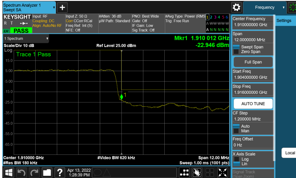
Plot 7-195. Upper Band Edge Plot (NR Band n2 - 15MHz QPSK – Full RB)
