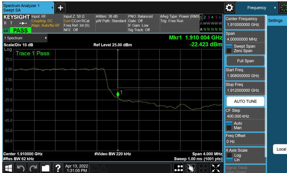
Plot 7-207. Upper Band Edge Plot (NR Band n2 – 5MHz QPSK – Full RB)
