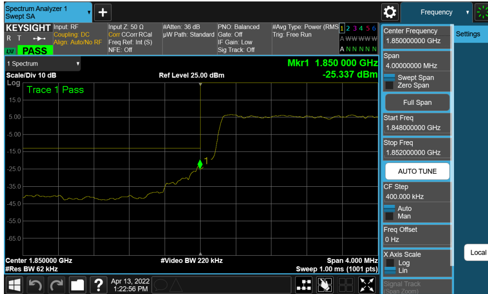
Plot 7-205. Lower Band Edge Plot (NR Band n25/2 – 5MHz QPSK – Full RB)
