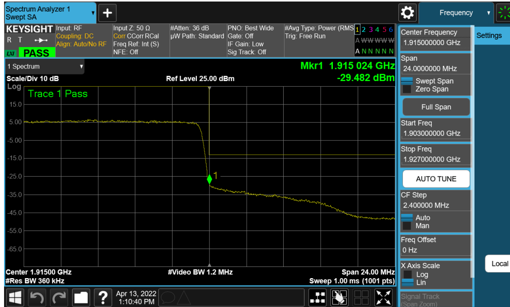
Plot 7-181. Upper Band Edge Plot (NR Band n25 - 30MHz QPSK – Full RB)
