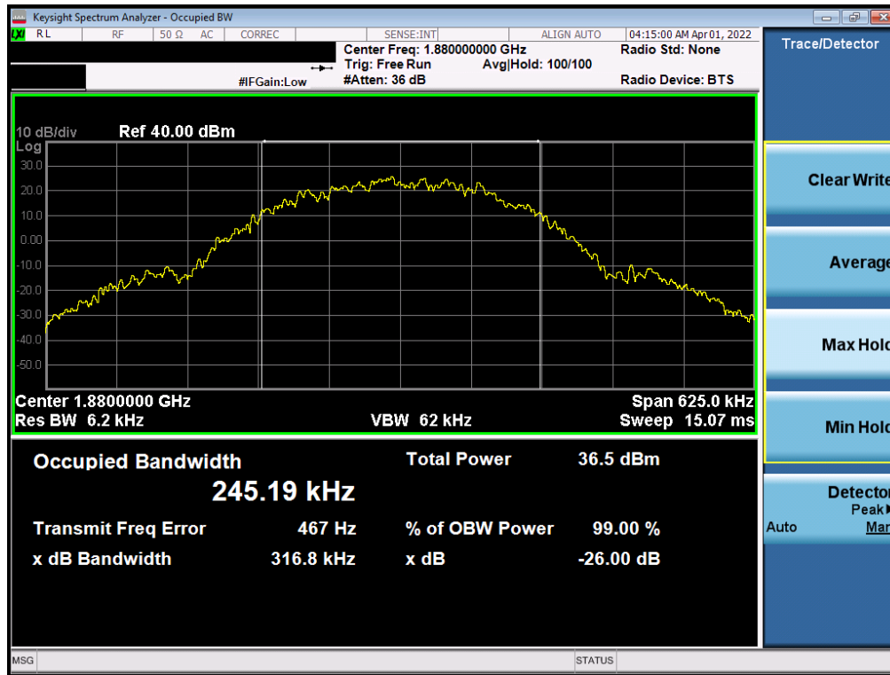
Plot 7-55. Occupied Bandwidth Plot (GPRS, Ch. 661)
