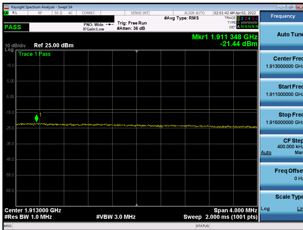
Plot 7-106. Extended Upper Band Edge Plot (LTE Band 2 - 20MHz QPSK – Full RB)
