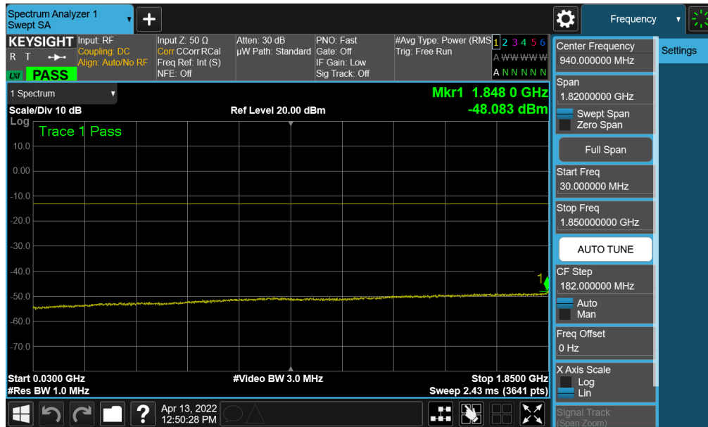
Plot 7-76. Conducted Spurious Plot (NR Band n25/2 - 20.0MHz - 1RB - Low Channel)
