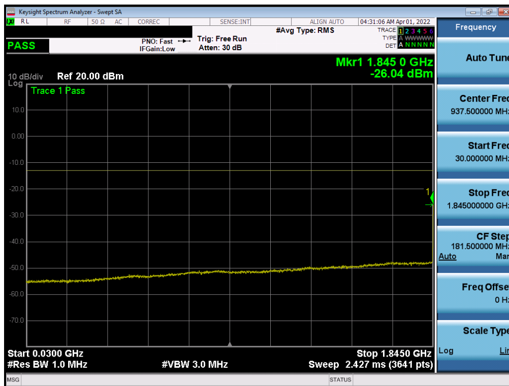
Plot 7-94. Conducted Spurious Plot (WCDMA Ch. 9262)
