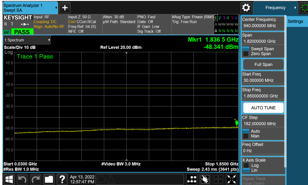
Plot 7-82. Conducted Spurious Plot (NR Band n25/2 - 20.0MHz - 1RB - High Channel)
