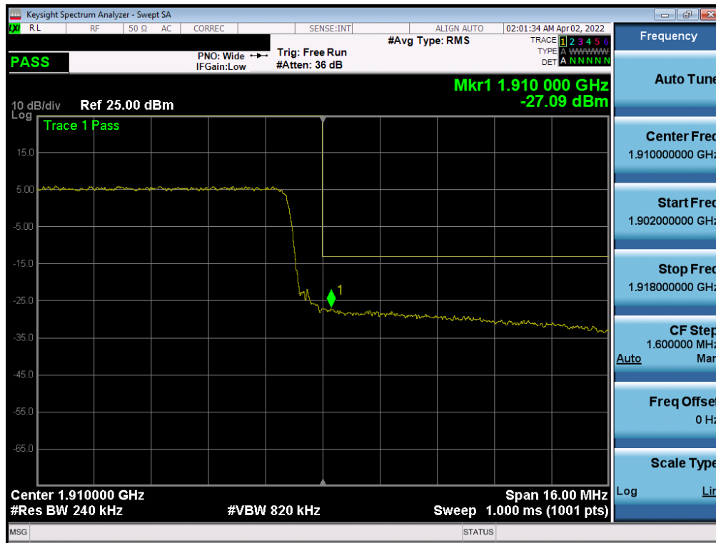
Plot 7-105. Upper Band Edge Plot (LTE Band 2 - 20MHz QPSK – Full RB)
