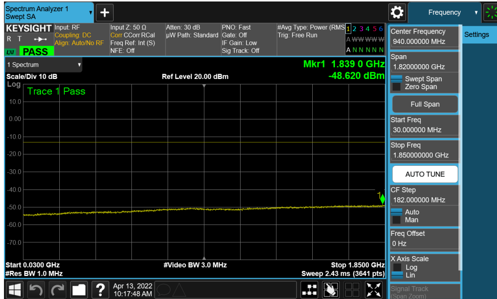
Plot 7-73. Conducted Spurious Plot (NR Band n25/2 - 20.0MHz - 1RB - High Channel)
