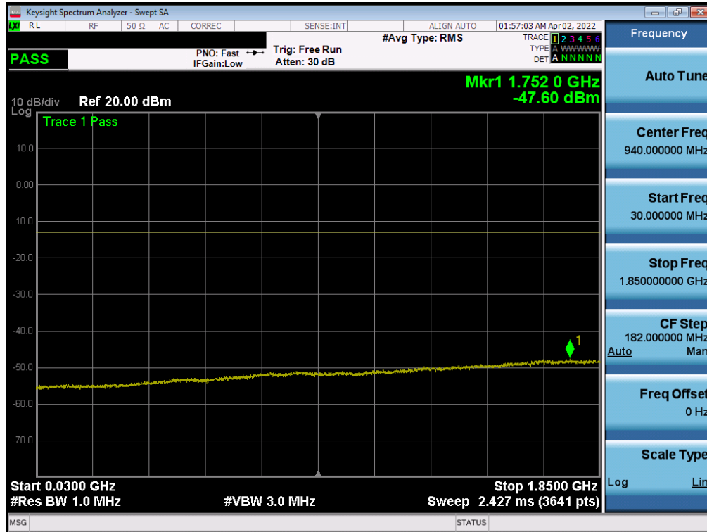
Plot 7-64. Conducted Spurious Plot (LTE Band 25/2 - 20MHz QPSK - 1RB - High Channel)
