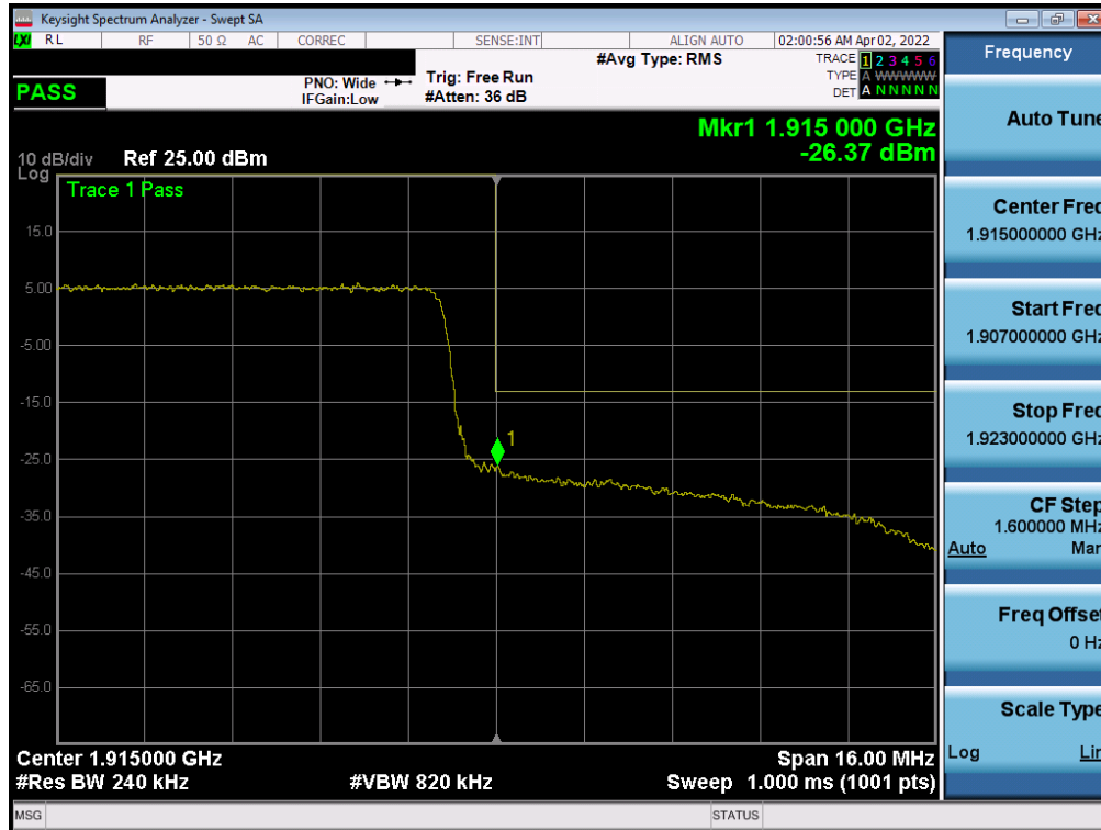
Plot 7-107. Upper Band Edge Plot (LTE Band 25 - 20MHz QPSK – Full RB)
