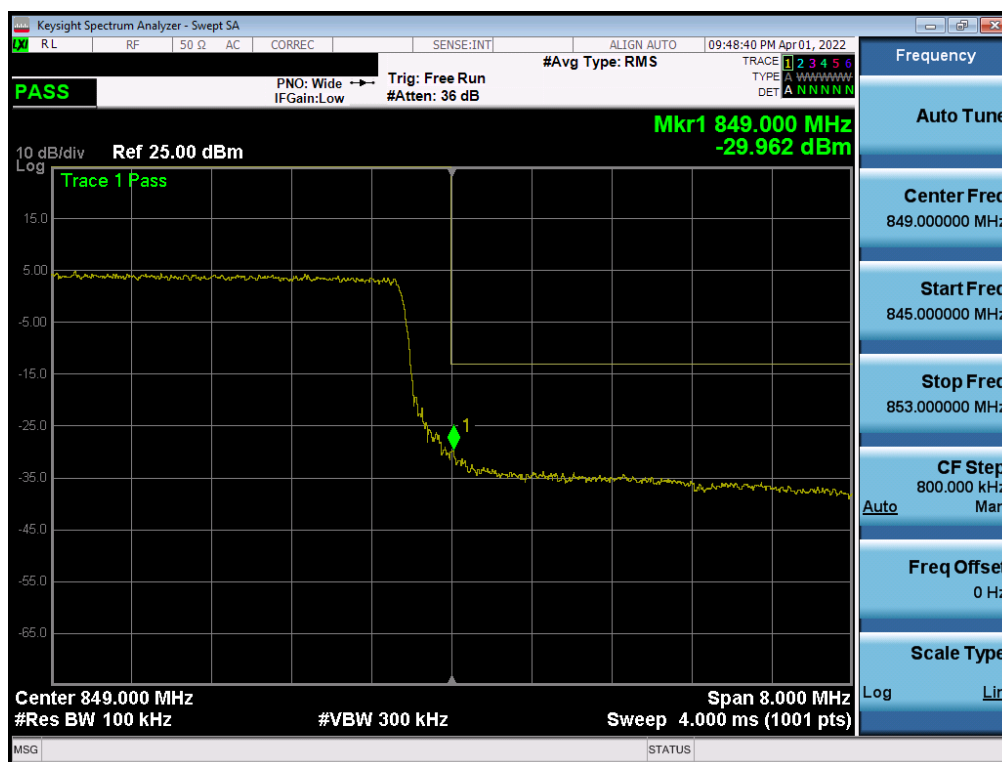
Plot 7-65. Upper Band Edge Plot (LTE Band 26/5 - 10MHz QPSK – Full RB)
