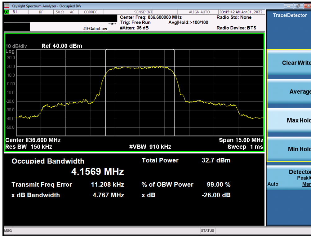
Plot 7-25. Occupied Bandwidth Plot (WCDMA, Ch. 4183)
