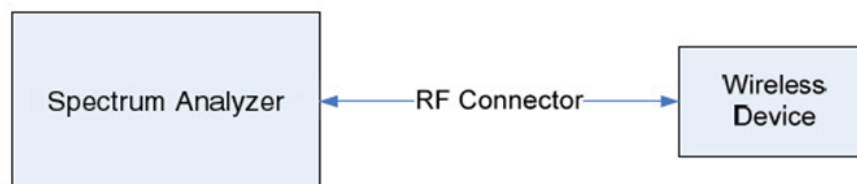
Figure 7-5. Test Instrument & Measurement Setup
