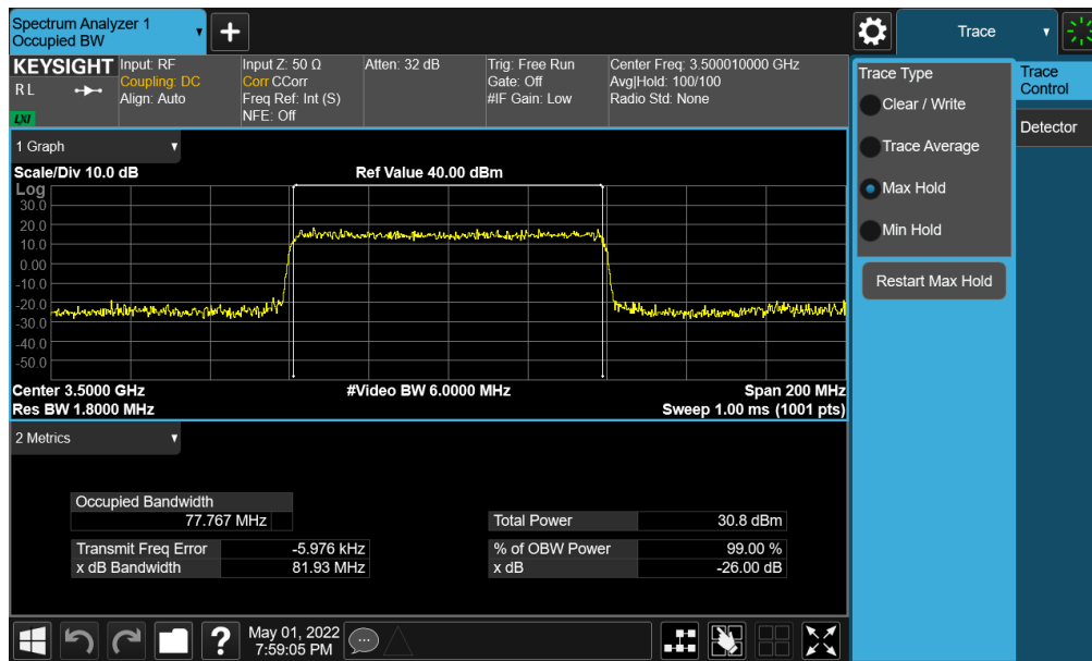
Plot 7-9. Occupied Bandwidth Plot (NR Band n77 - DoD Band – 80MHz – 16-QAM - Full RB)
