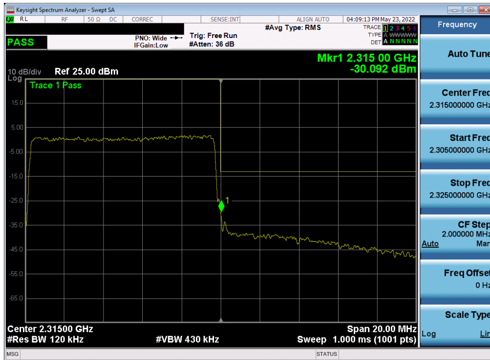
Plot 7-292. Upper Band Edge Plot (NR Band n30 - 10MHz - Full RB)
