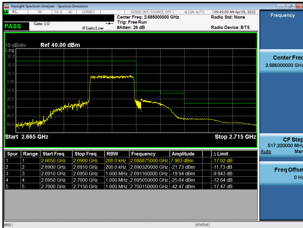
Plot 7-227. Upper ACP Plot (LTE Band 41(PC3) - 10MHz QPSK – Full RB)
