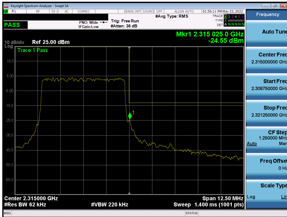
Plot 7-244. Upper Band Edge Plot (NR Band n30 - 5MHz - Full RB)
