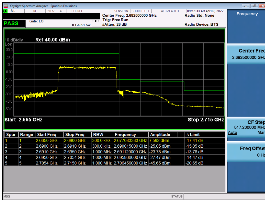
Plot 7-225. Upper ACP Plot (LTE Band 41(PC3) - 15MHz QPSK – Full RB)
