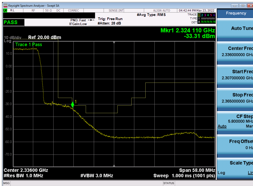
Plot 7-241. Extended Upper Band Edge Plot (NR Band n30 - 10MHz – Full RB)
