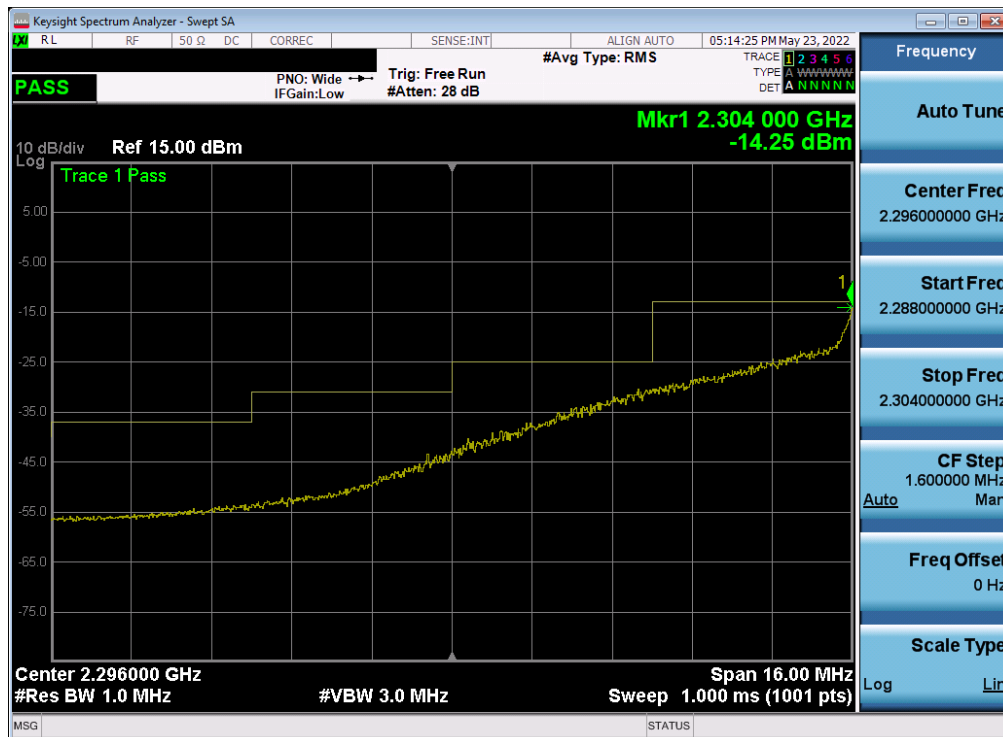
Plot 7-243. Extended Lower Band Edge Plot (NR Band n30 - 5MHz - Full RB)
