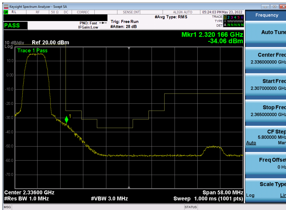
Plot 7-245. Extended Upper Band Edge Plot (NR Band n30 - 5MHz - Full RB)
