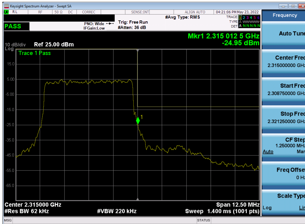
Plot 7-296. Upper Band Edge Plot (NR Band n30 - 5MHz - Full RB)
