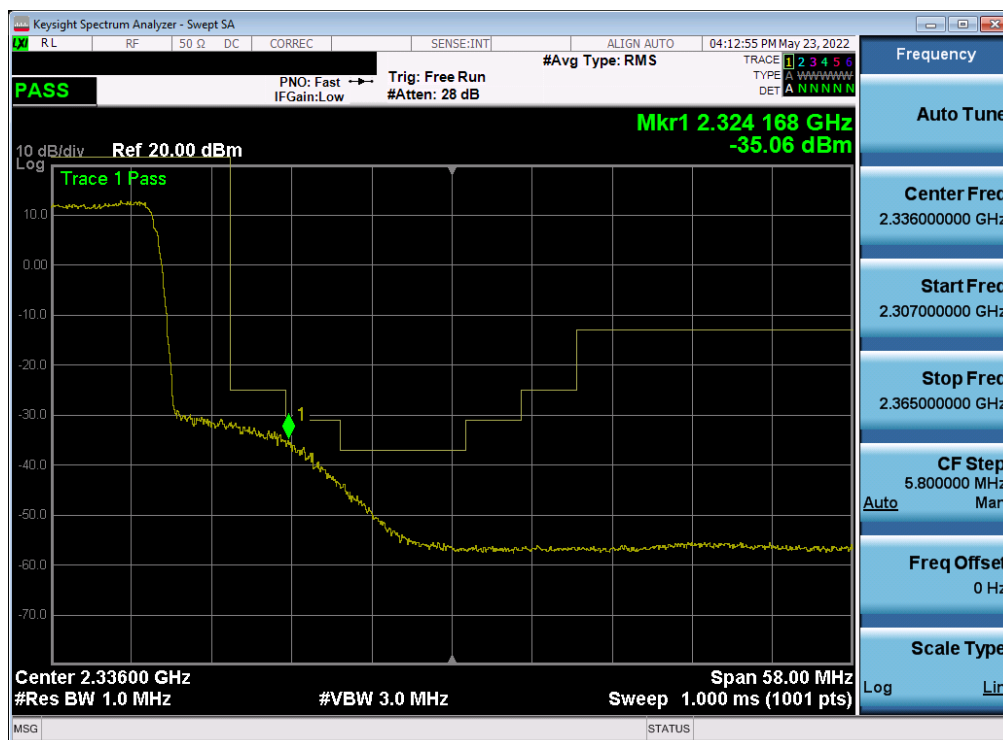
Plot 7-293. Extended Upper Band Edge Plot (NR Band n30 - 10MHz - Full RB)
