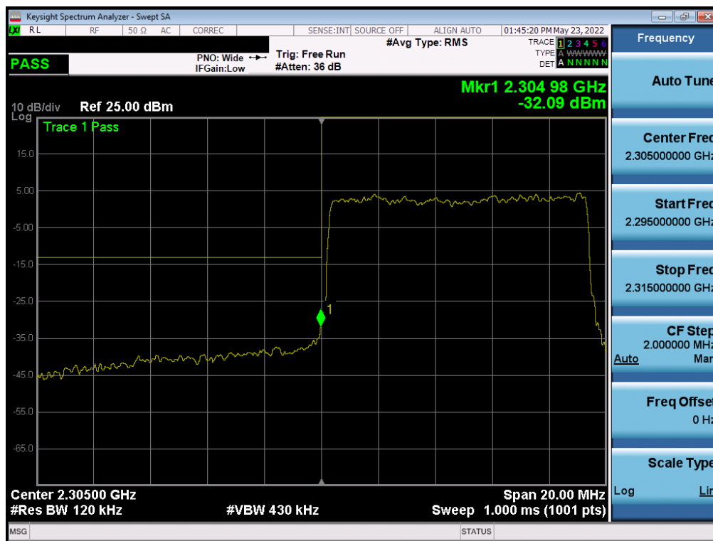
Plot 7-238. Lower Band Edge Plot (NR Band n30 - 10MHz - Full RB)
