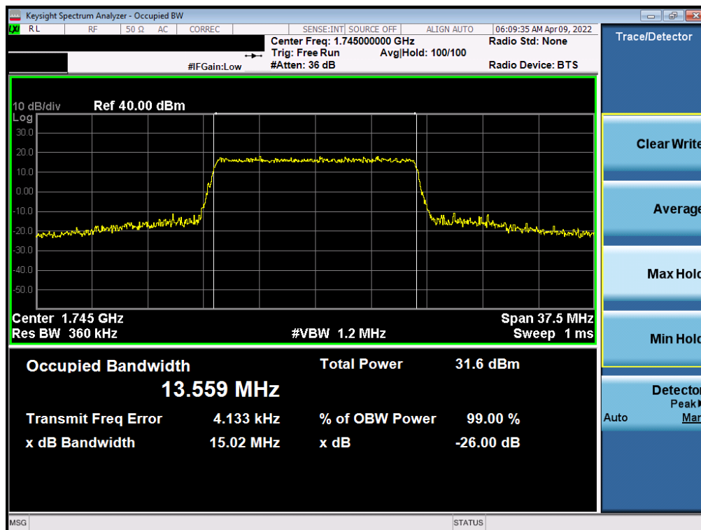
Plot 7-46. Occupied Bandwidth Plot (LTE Band 66/4 - 15MHz 16-QAM - Full RB)
