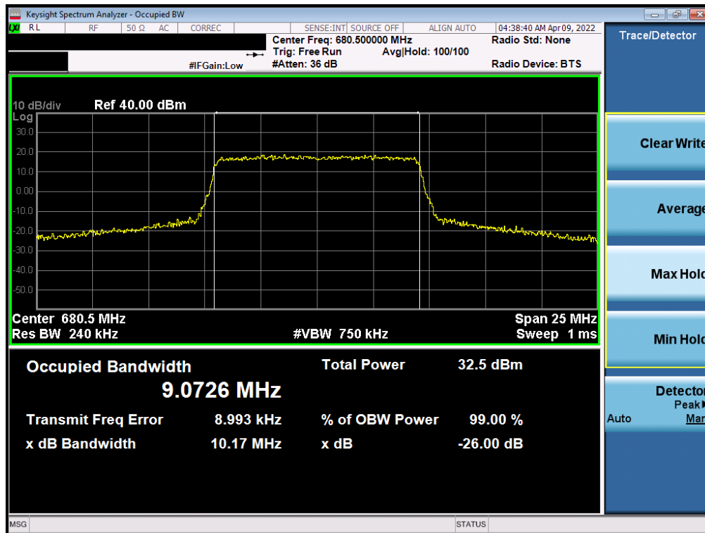
Plot 7-5. Occupied Bandwidth Plot (LTE Band 71 - 10MHz QPSK - Full RB)
