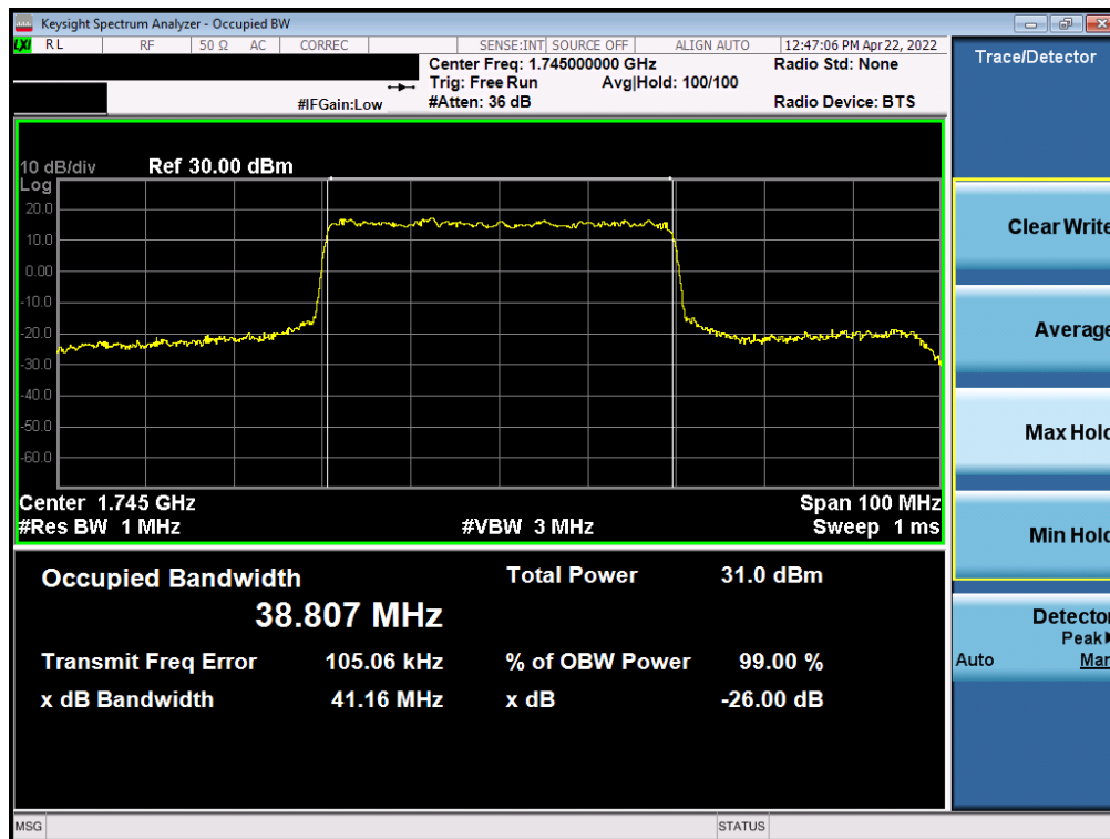
Plot 7-56. Occupied Bandwidth Plot (NR Band n66 - 40.0MHz CP-OFDM QPSK - Full RB)
