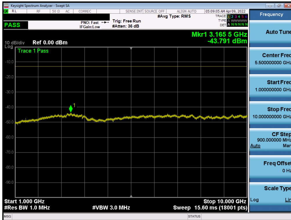
Plot 7-105. Conducted Spurious Plot (LTE Band 12 - 10MHz QPSK - 1 RB - Mid Channel)
