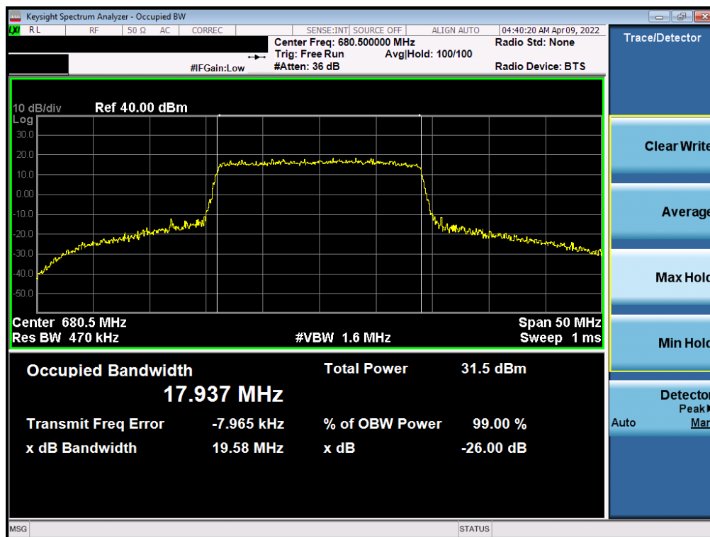
Plot 7-2. Occupied Bandwidth Plot (LTE Band 71 - 20MHz 16-QAM - Full RB)
