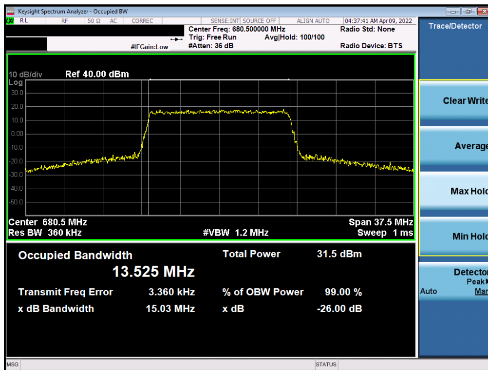
Plot 7-4. Occupied Bandwidth Plot (LTE Band 71 - 15MHz 16-QAM - Full RB)
