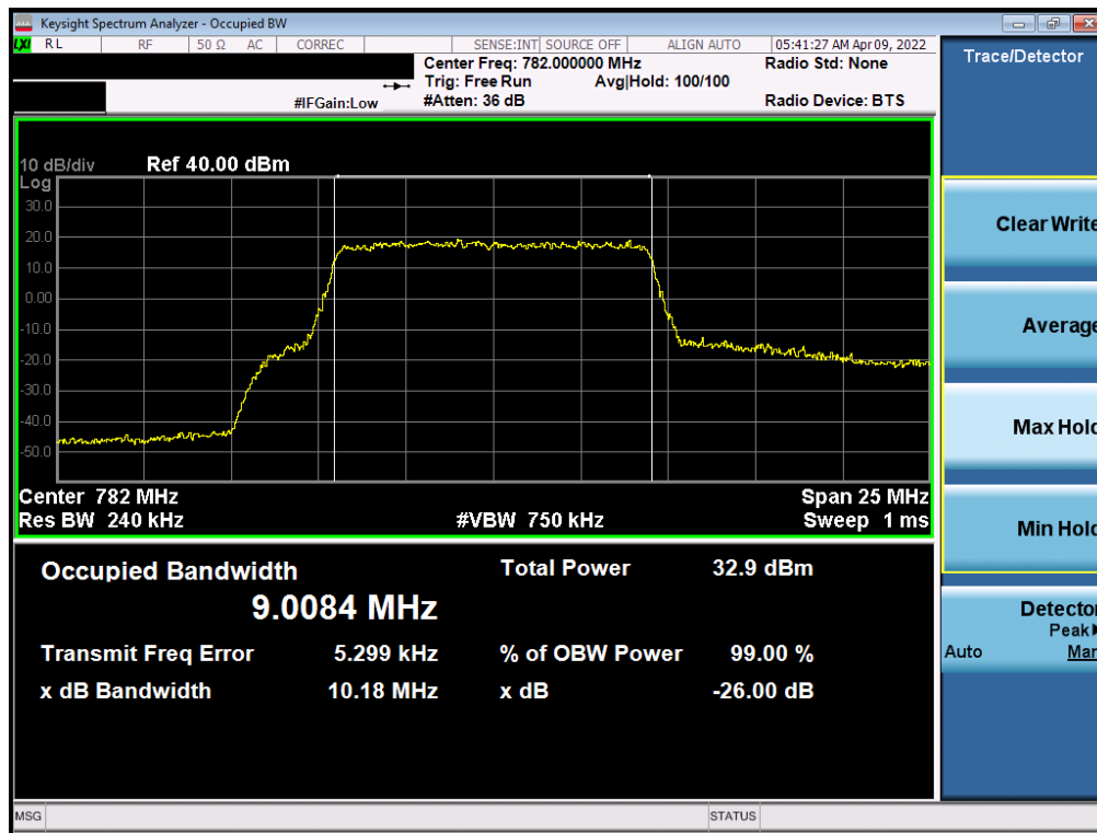
Plot 7-17. Occupied Bandwidth Plot (LTE Band 13 - 10MHz QPSK - Full RB)
