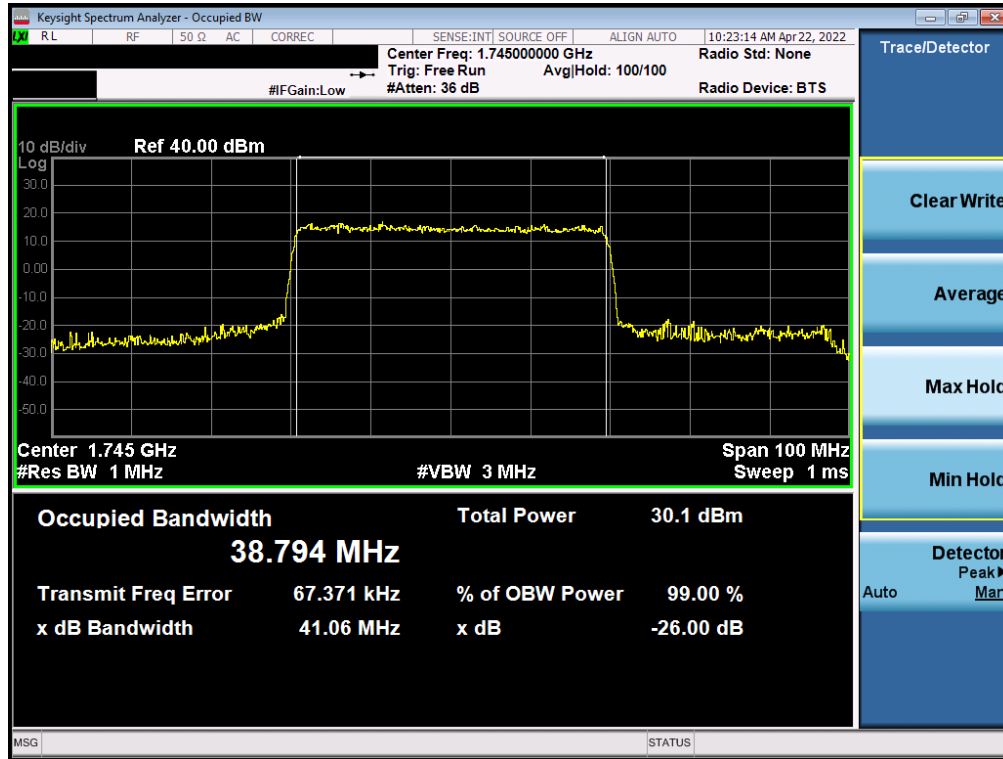
Plot 7-75. Occupied Bandwidth Plot (NR Band n66 - 40.0MHz CP-OFDM 16QAM - Full RB)
