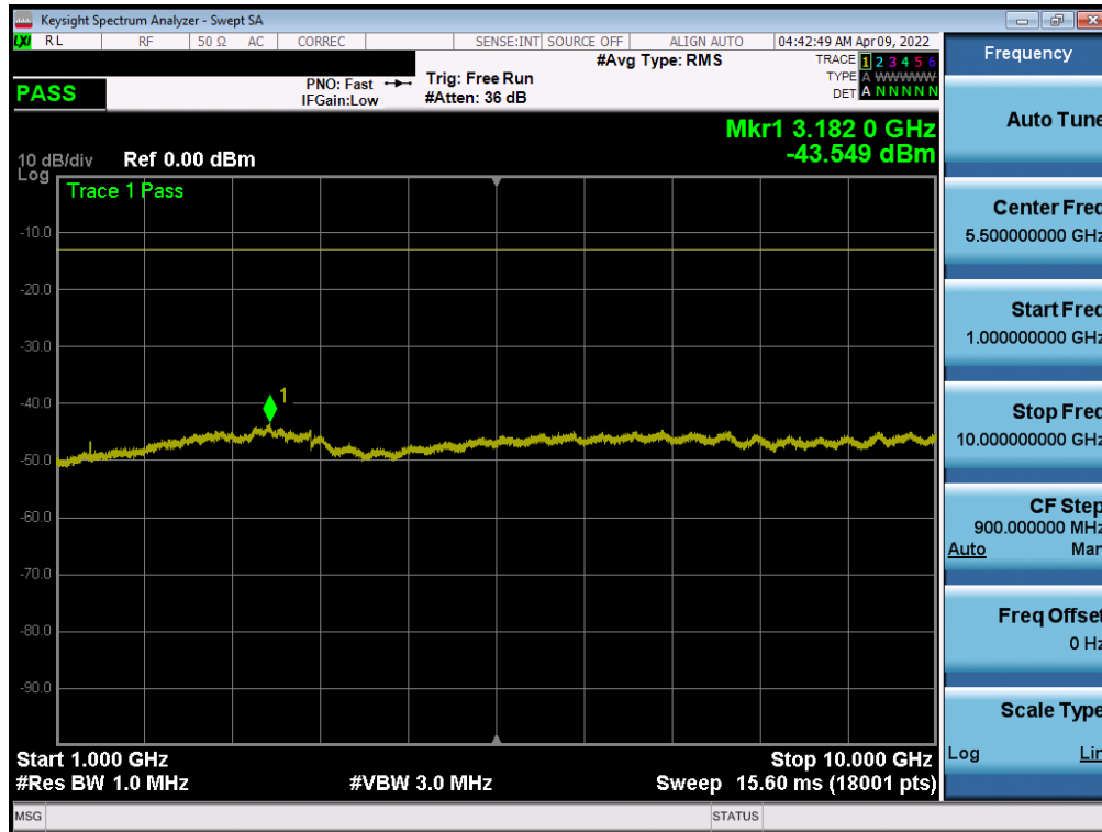
Plot 7-93. Conducted Spurious Plot (LTE Band 71 - 20MHz QPSK - 1 RB - Low Channel)
