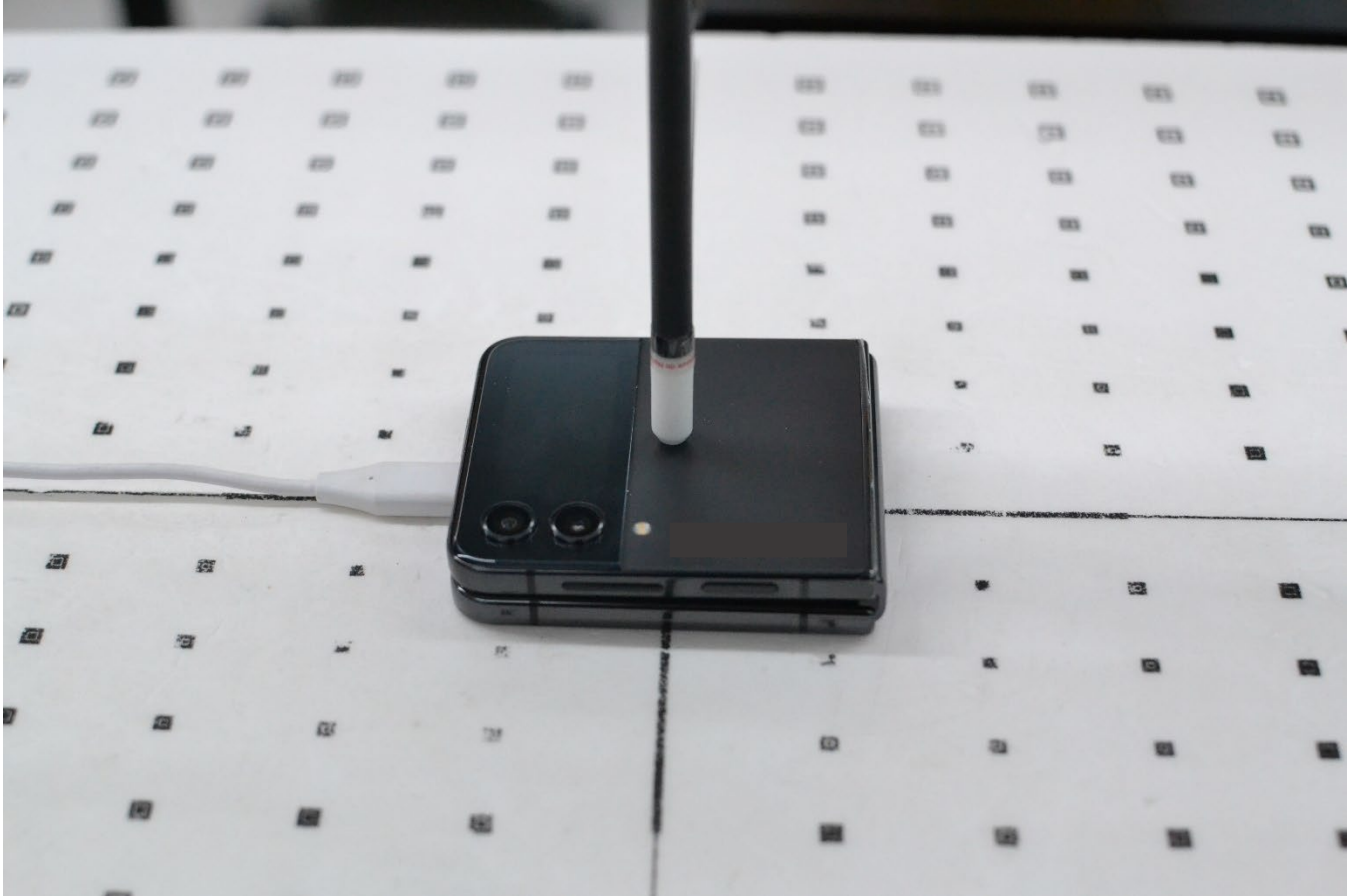
Figure E-5 Near Field Power Density Test Setup Photo – Front Side Closed at 2 mm
