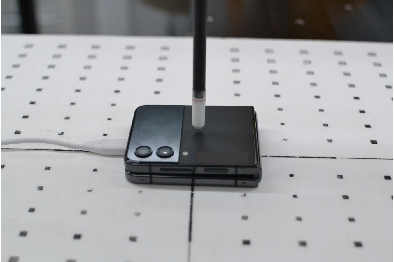
Figure E-6 Near Field Power Density Test Setup Photo – Front Side Closed at 5 mm
