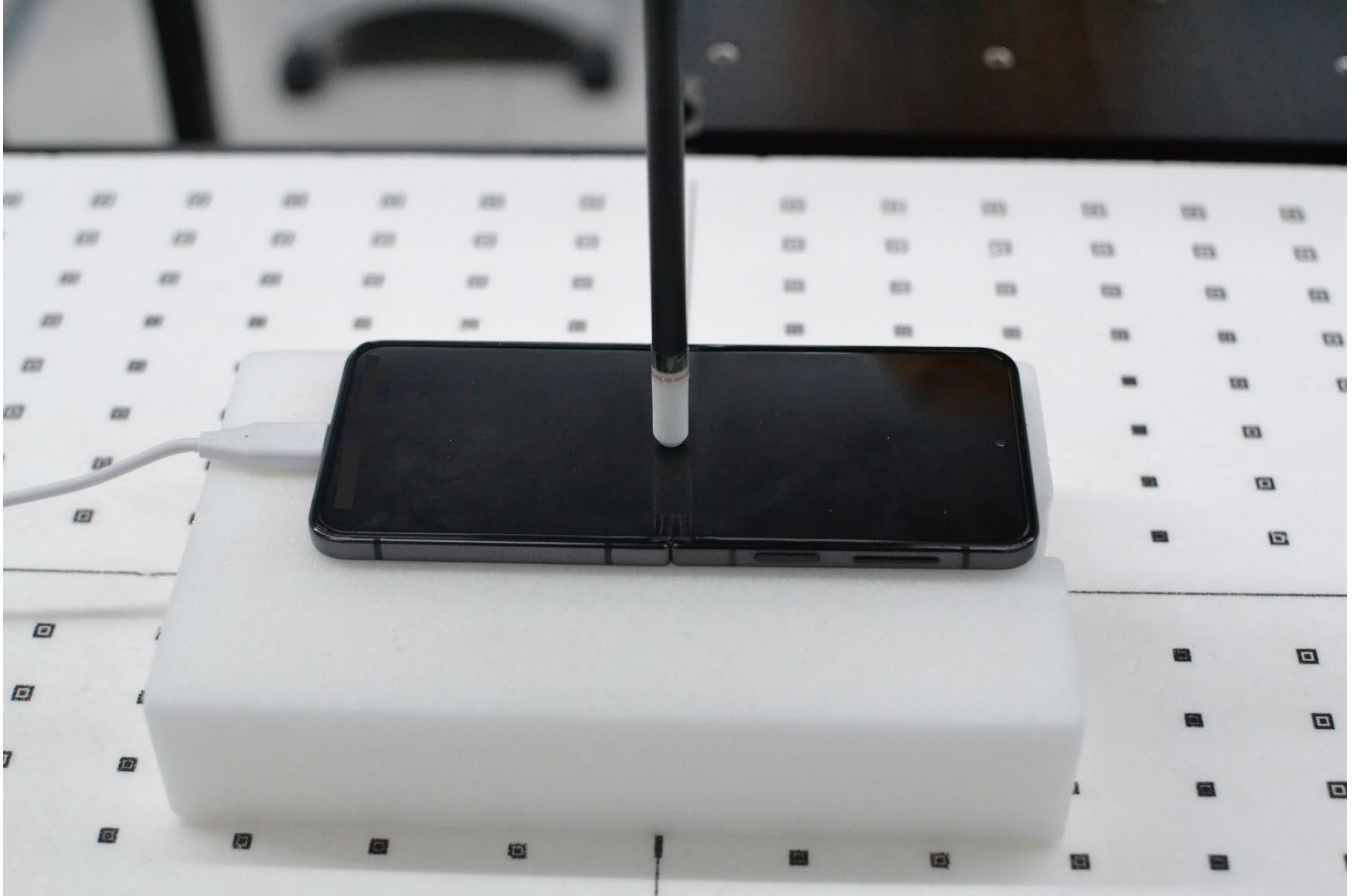
Figure E-7 Near Field Power Density Test Setup Photo – Front Side Open at 2 mm
