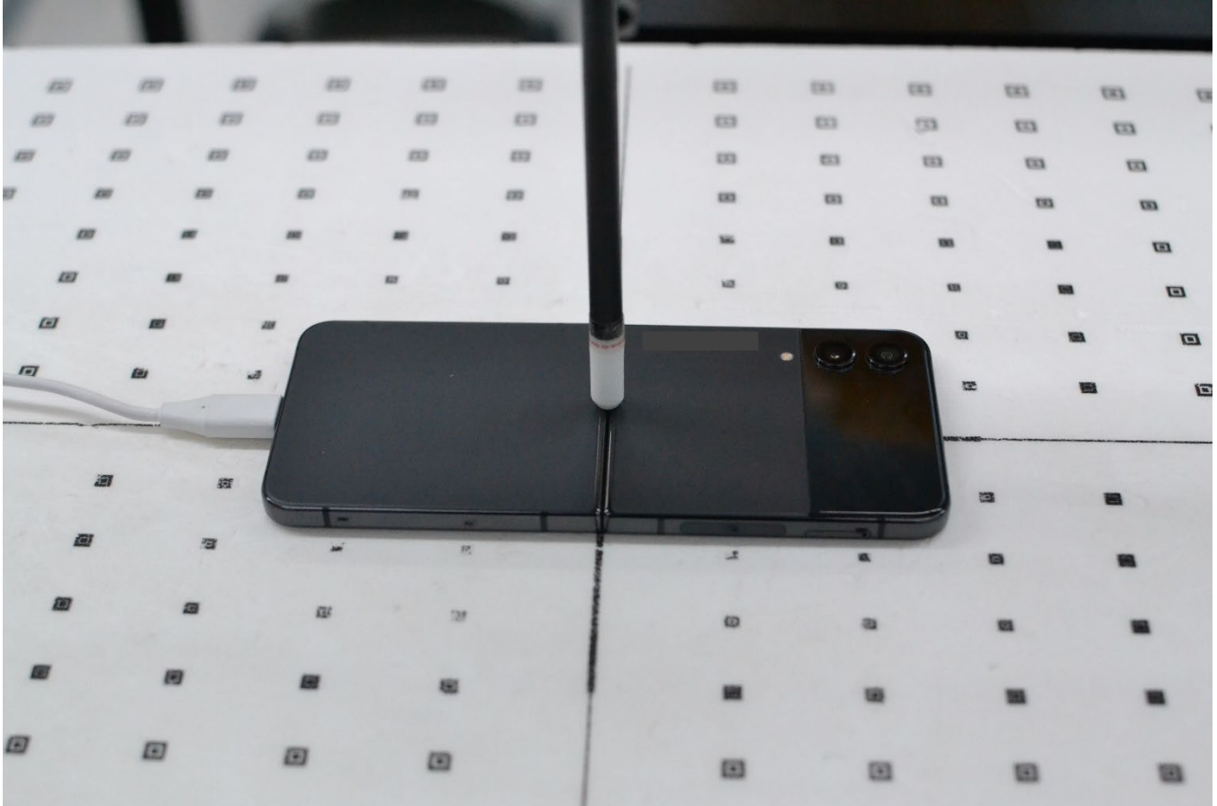
Figure E-4 Near Field Power Density Test Setup Photo – Back Side Open at 2 mm
