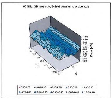
Probe isotropy for E<sub>tot</sub>: probe rotated  $\phi$  = 0° to 360°, tilted from field propagation direction  $\vec{k}$  Parallel to the field propagation ( $\psi$  =0° - 90°) at 30 GHz: deviation within ± 0.36 dB Parallel to the field propagation ( $\psi$  =0° - 90°) at 60 GHz: deviation within ± 0.33 dB
