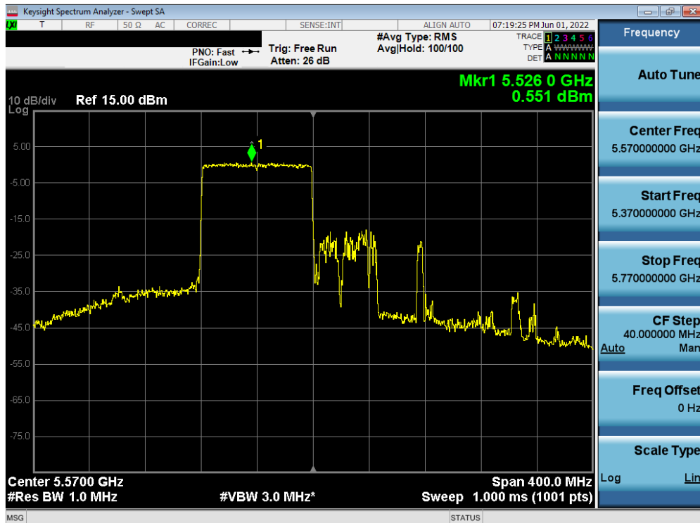
Plot 7-219. Power Spectral Density Plot SISO ANT1 (160MHz L BW 802.11ax – Full Tones (UNII Band 2C) – Ch. 138)
