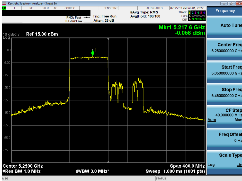
Plot 7-202. Power Spectral Density Plot SISO ANT1 (160MHz L BW 802.11ax – Full Tones (UNII Band 1/2A) – Ch. 50)
