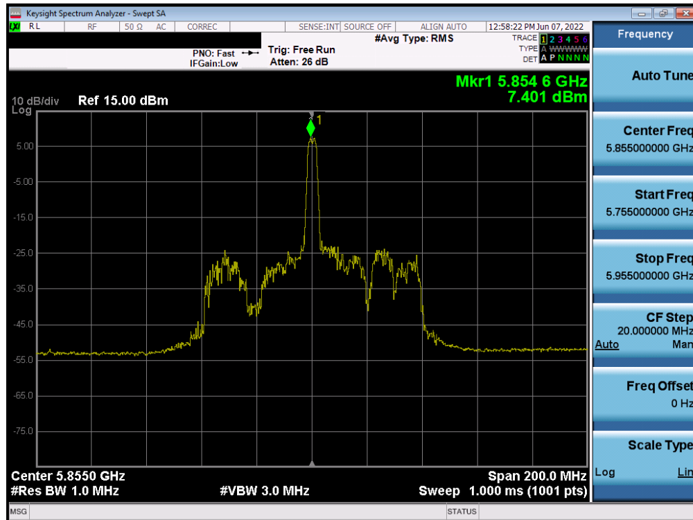
Plot 7-193. Power Spectral Density Plot SISO ANT1 (80MHz BW 802.11ax – 26 Tones (UNII Band 3/4) – Ch. 171)
