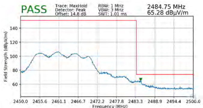
Plot 7-136. Radiated Restricted Upper Band Edge Measurement MIMO (Peak)
