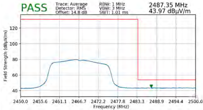
Plot 7-121. Radiated Restricted Upper Band Edge Measurement SISO ANT1 (Average)
