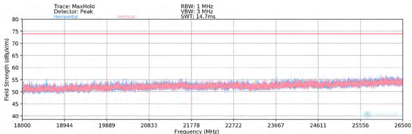
Plot 7-100. Radiated Spurious Plot above 18GHz SISO ANT1 – Half Open
