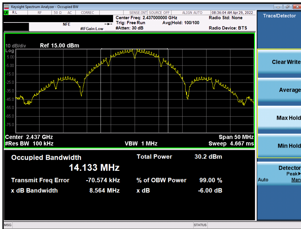
Plot 7-14. 6dB Bandwidth Plot SISO ANT2 (802.11b – Ch. 6)
