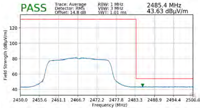
Plot 7-129. Radiated Restricted Upper Band Edge Measurement SISO ANT2 (Average)
