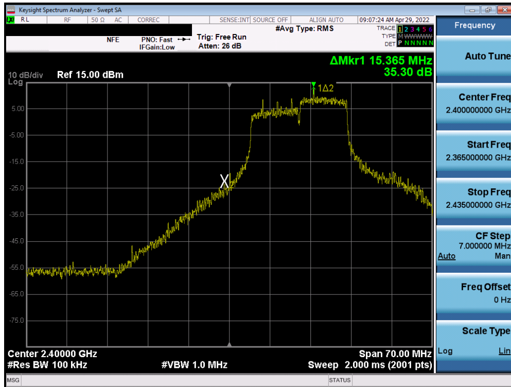
Plot 7-69. Band Edge Plot SISO ANT2 (802.11g- Ch. 1)
