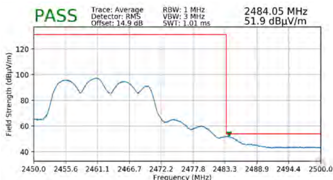
Plot 7-135. Radiated Restricted Upper Band Edge Measurement MIMO (Average)
