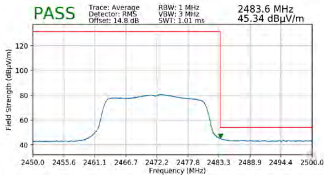
Plot 7-123. Radiated Restricted Upper Band Edge Measurement SISO ANT1 (Average)
