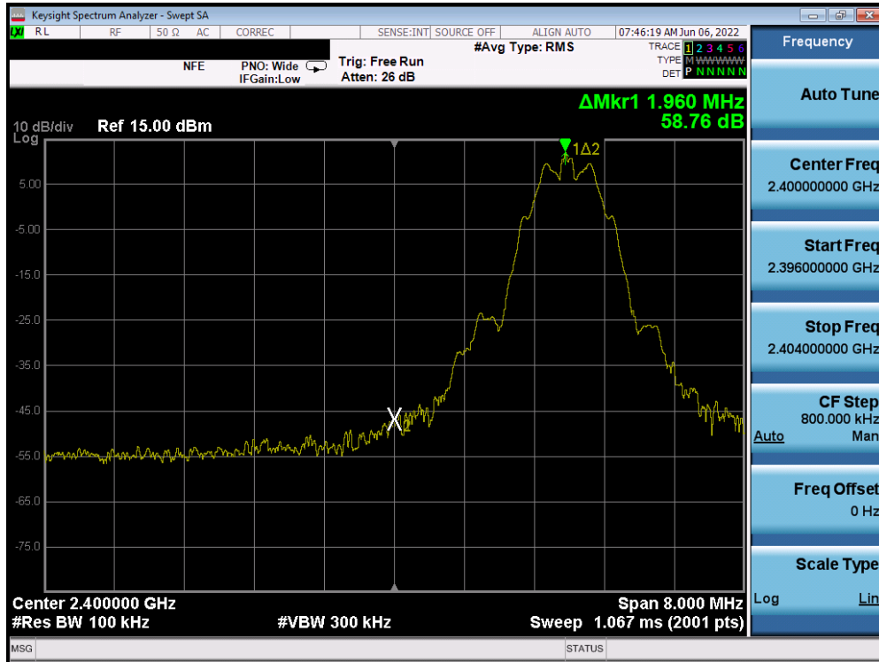
Plot 7-83. Band Edge Plot (Bluetooth (LE), 500kbps – Ch. 0) – ANT 2
