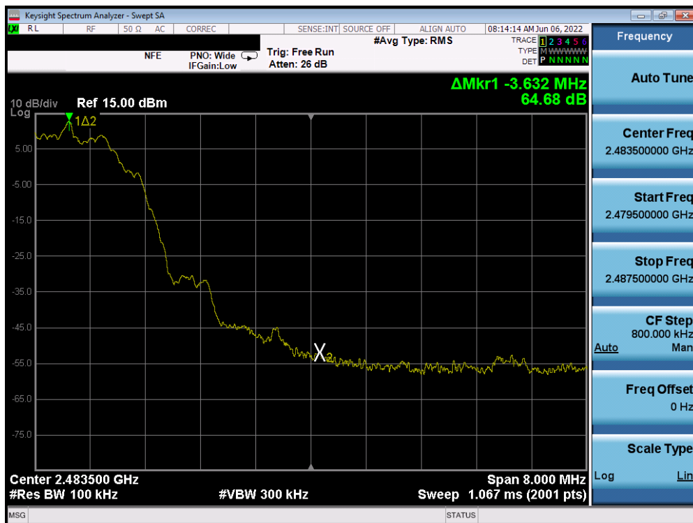
Plot 7-88. Band Edge Plot (Bluetooth (LE), 2Mbps – Ch. 39) – ANT 2
