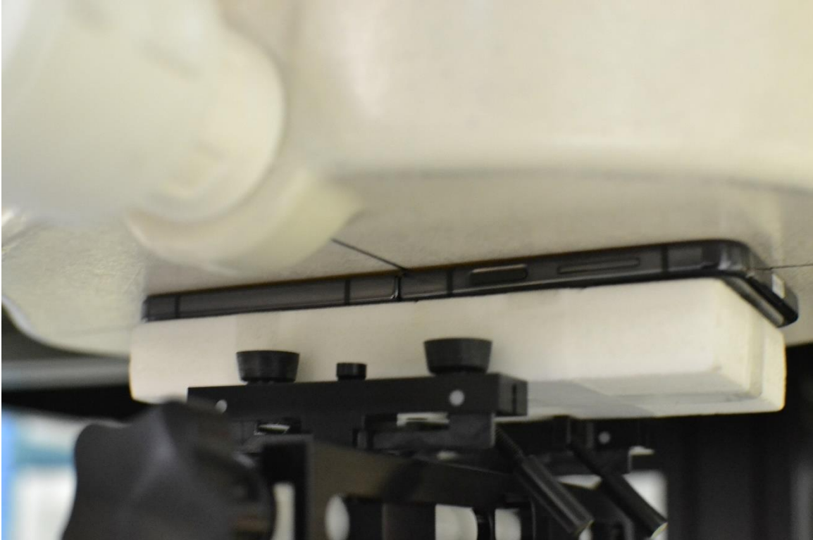
SAR Test Setup Photo 11 – Phablet, Front Side at 0 mm
