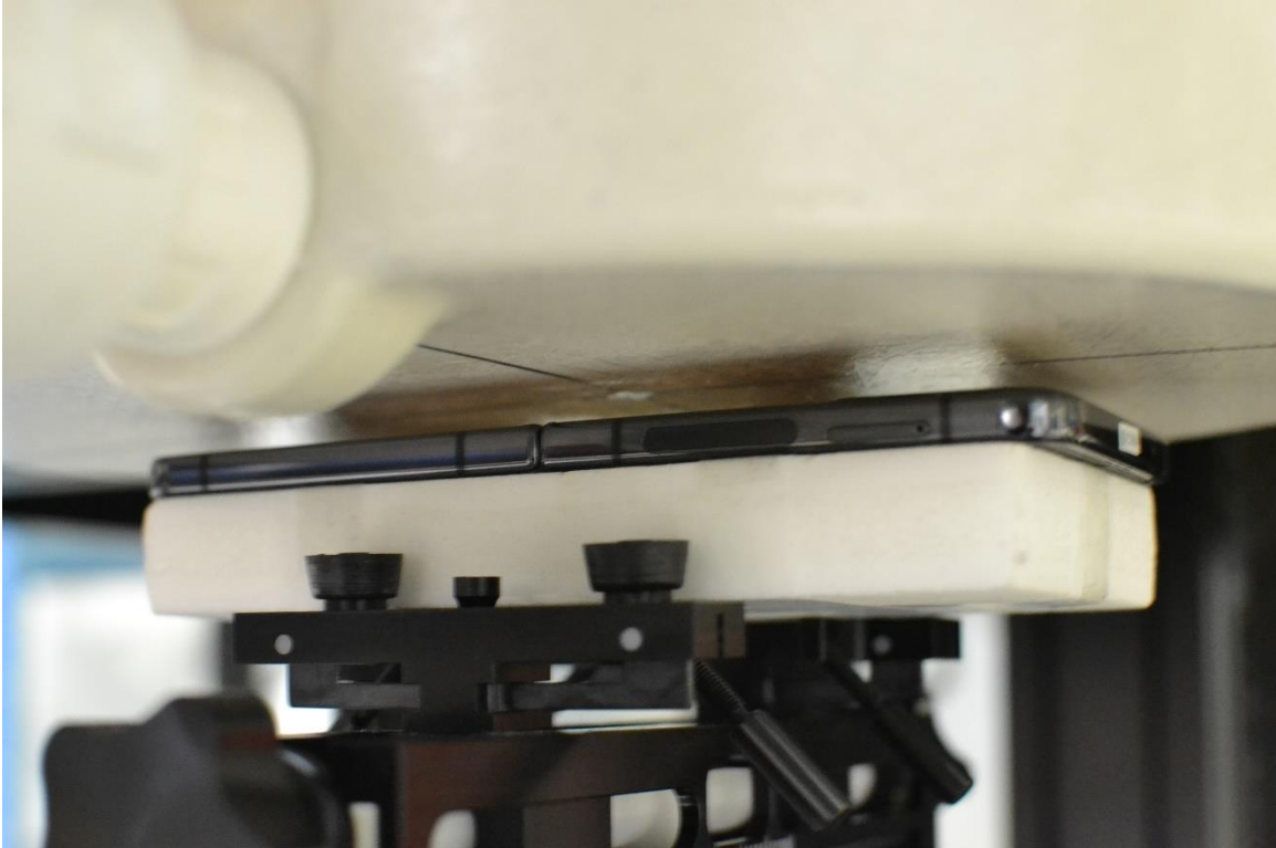
SAR Test Setup Photo 7 – Phablet, Back Side at 8 mm
