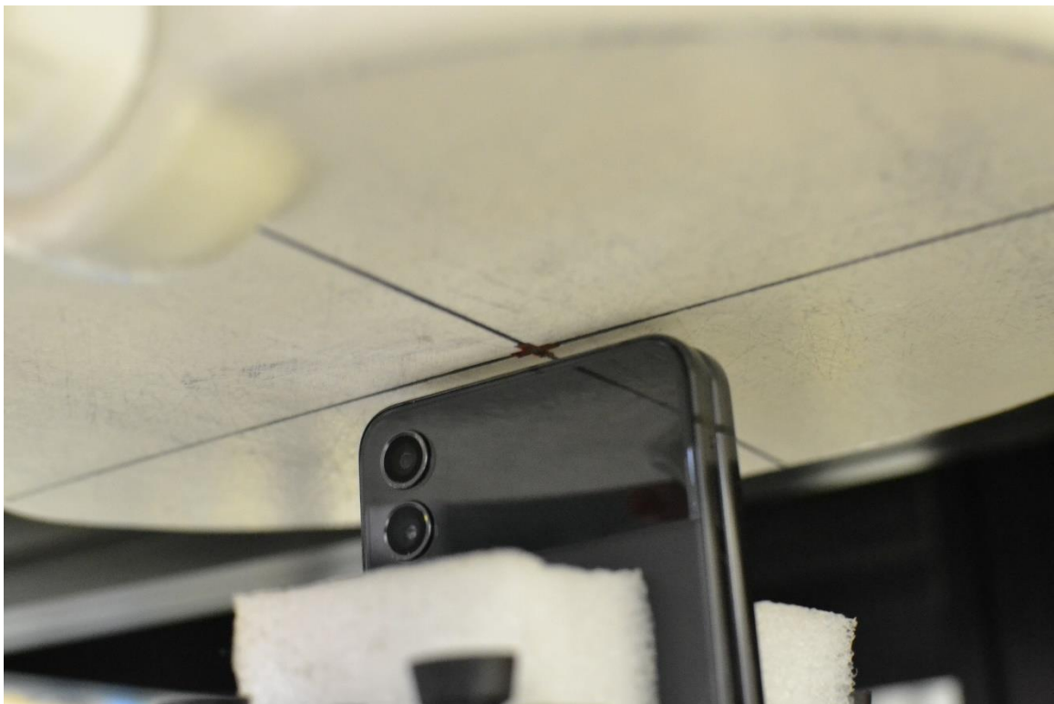
SAR Test Setup Photo 25 – Closed Hotspot, Bottom Edge at 5 mm
