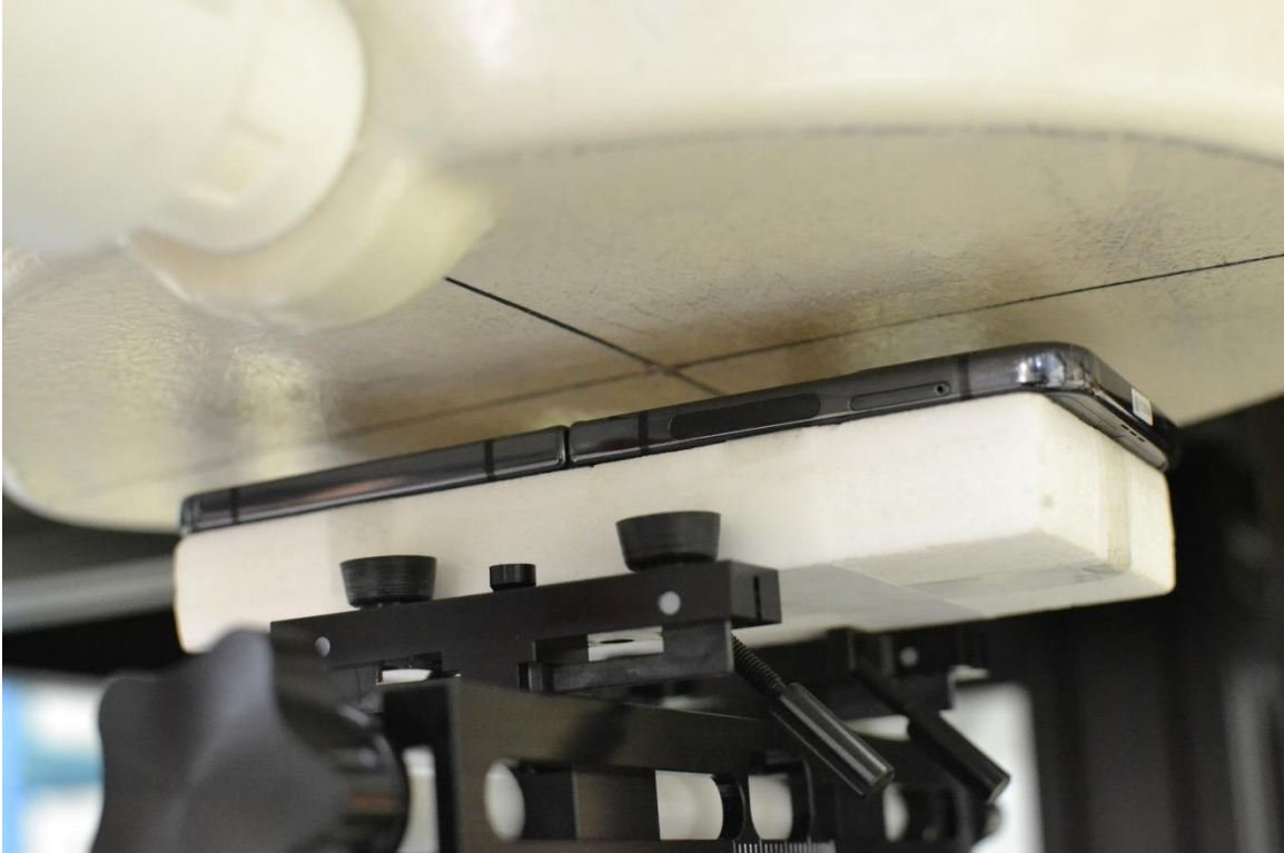
SAR Test Setup Photo 5 – Body-worn, Back Side at 15 mm
