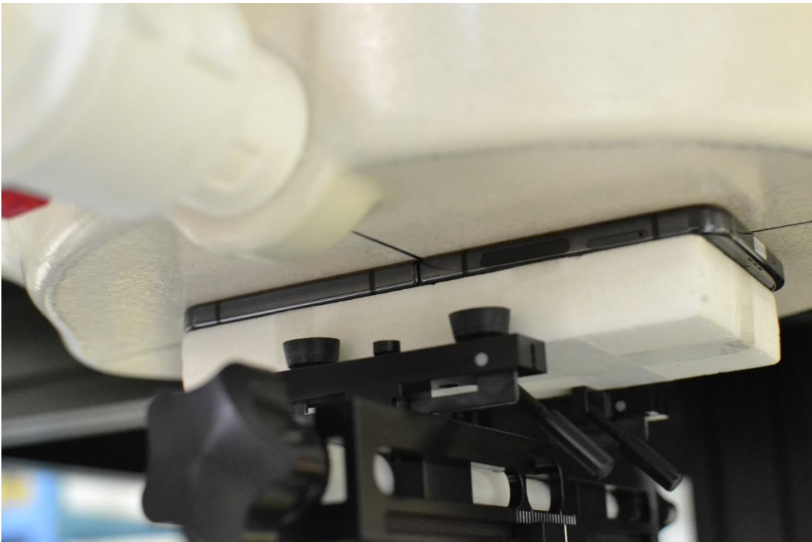
SAR Test Setup Photo 8 – Phablet, Back Side at 0 mm
