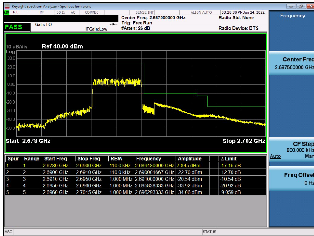
Plot 7-35. Upper ACP Plot (LTE Band 41(PC3) - 5MHz QPSK – Full RB)
