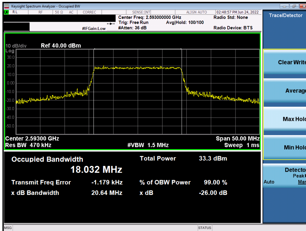
Plot 7-3. Occupied Bandwidth Plot (LTE Band 41(PC3) - 20MHz 16-QAM - Full RB)
