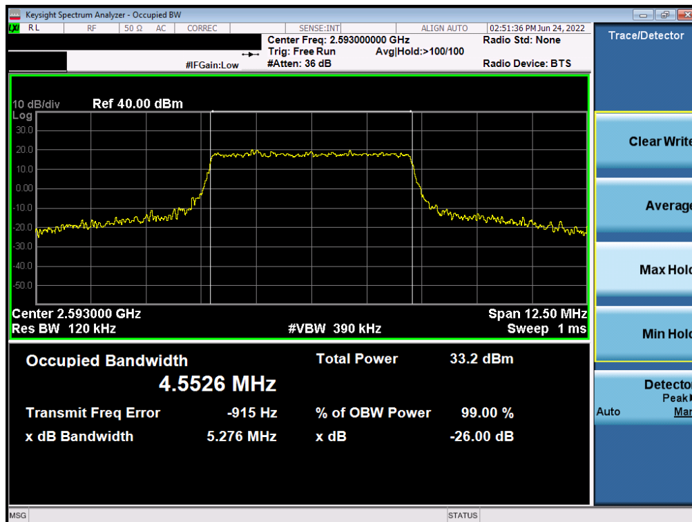
Plot 7-9. Occupied Bandwidth Plot (LTE Band 41(PC3) - 5MHz 16-QAM - Full RB)
