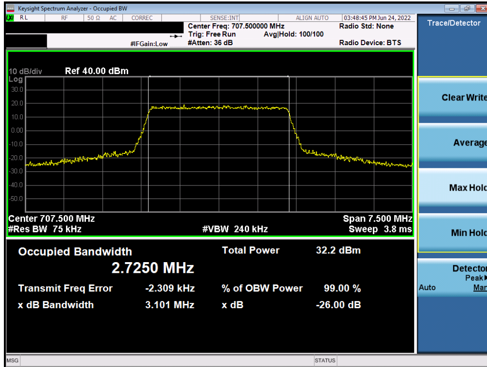
Plot 7-5. Occupied Bandwidth Plot (LTE Band 12 - 3MHz QPSK - Full RB)
