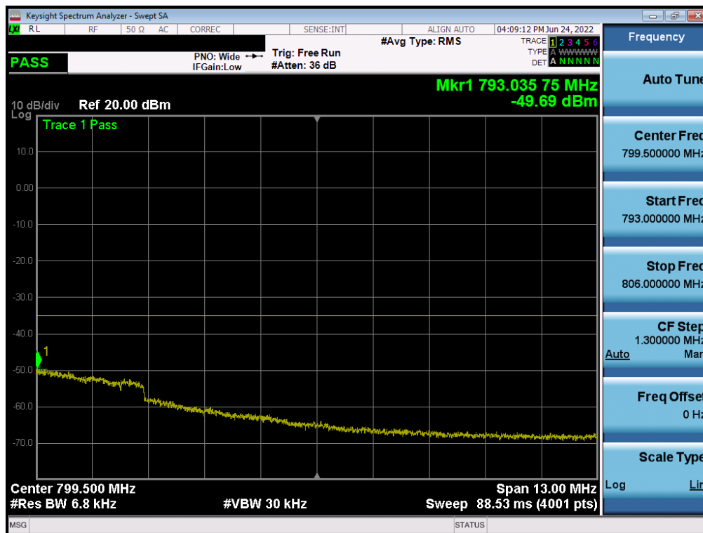
Plot 7-57. Upper Emission Mask Plot (LTE Band 13 – 10MHz QPSK – Full RB)
