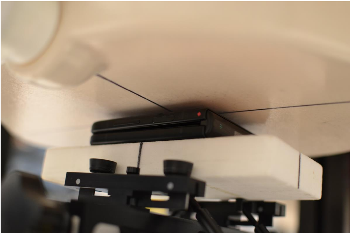
SAR Test Setup Photo 13 – Closed Hotspot, Back Side, 5 mm
