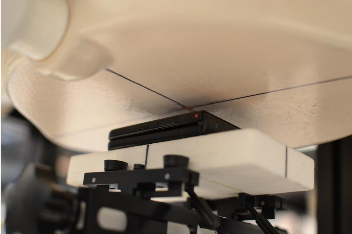
SAR Test Setup Photo 12 – Closed Body-Worn Back Side, 15 mm
