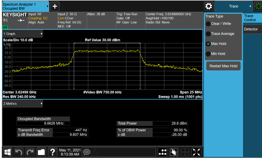
Plot 7-9. Occupied Bandwidth Plot (NR Band n48 - 10MHz 16-QAM - Full RB Configuration)
