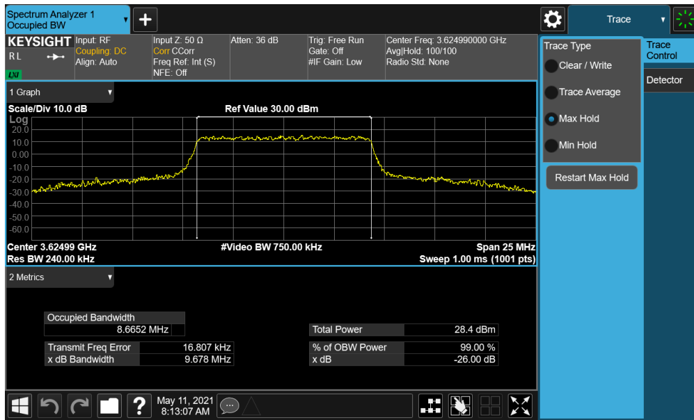
Plot 7-8. Occupied Bandwidth Plot (NR Band n48 - 10MHz QPSK - Full RB Configuration)
