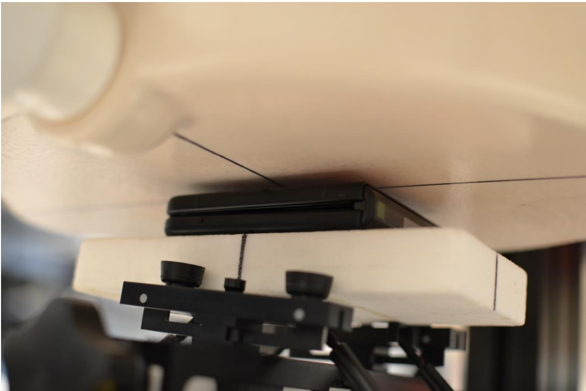
SAR Test Setup Photo 23 – Closed Hotspot, Back Side, 5 mm
