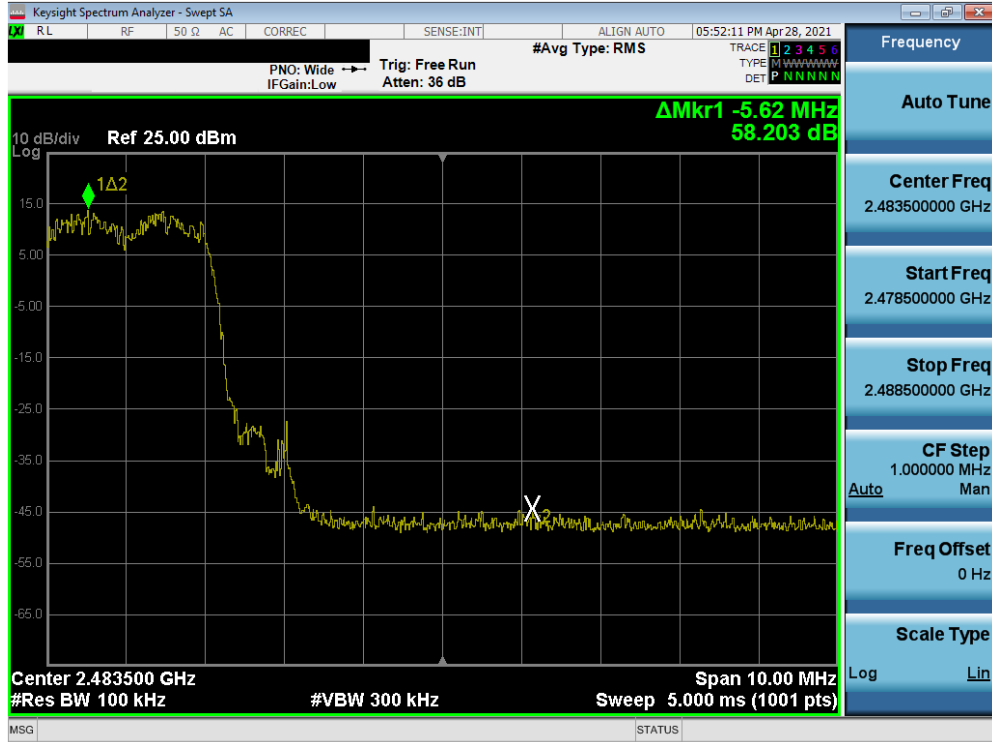
Plot 7-120. Band Edge Plot (Bluetooth with Hopping Enabled, ePA, 3 Mbps – Ch.78) – ANT1
