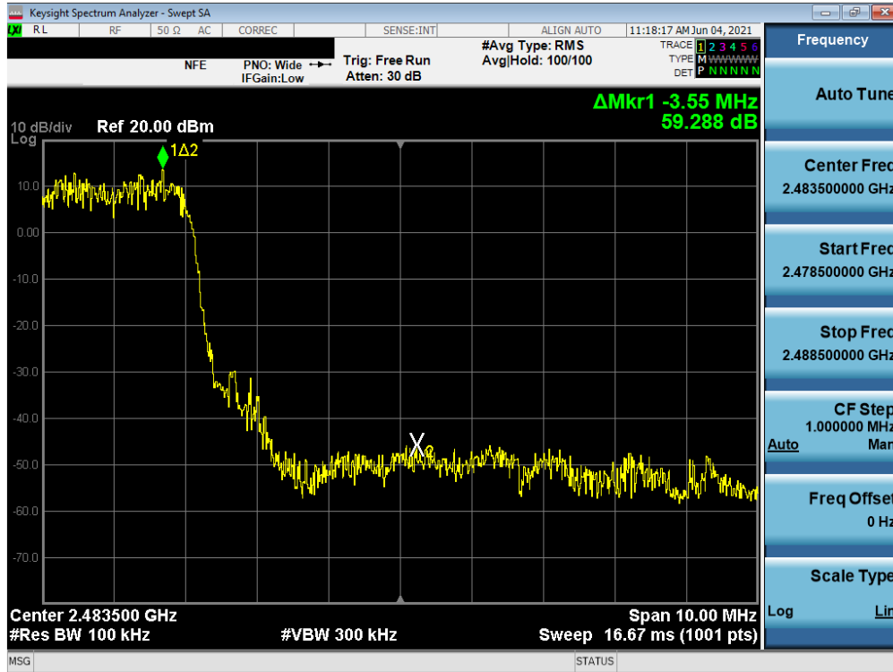
Plot 7-124. Band Edge Plot (Bluetooth with Hopping Enabled, iPA, 3 Mbps – Ch.78) – ANT1
