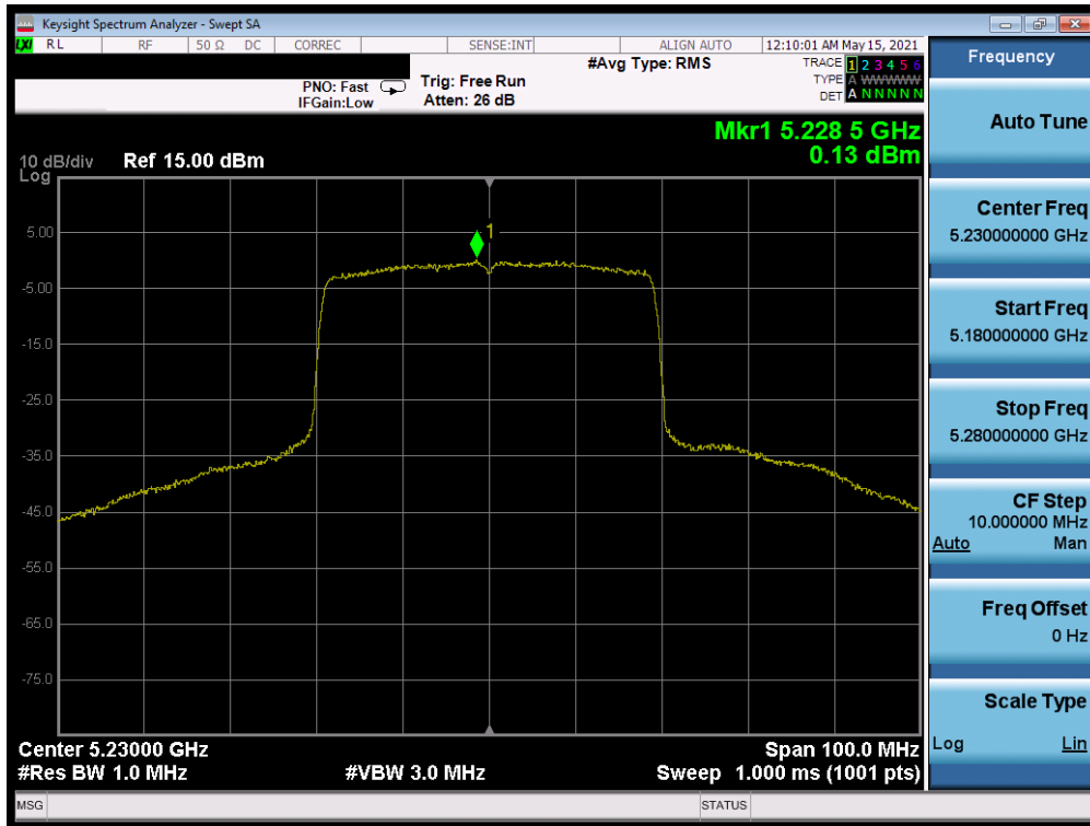
Plot 7-261. Power Spectral Density Plot MIMO ANT2 (40MHz BW 802.11ax (UNII Band 1) – Ch. 46)
