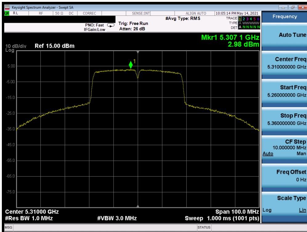
Plot 7-223. Power Spectral Density Plot MIMO ANT1 (40MHz BW 802.11n (UNII Band 2A) – Ch. 62)
