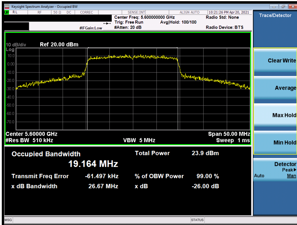
Plot 7-38. 26dB Bandwidth Plot ANT1 (20MHz BW 802.11ax (UNII Band 2C) – Ch. 120)
