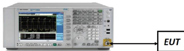
Figure 7-1. Test Instrument & Measurement Setup
