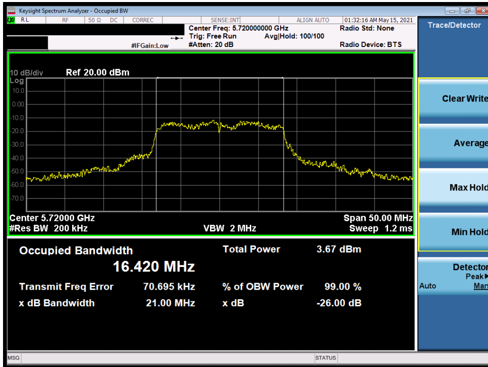
Plot 7-84. 26dB Bandwidth Plot MIMO (20MHz BW 802.11a (UNII Band 2C) – Ch. 144)
