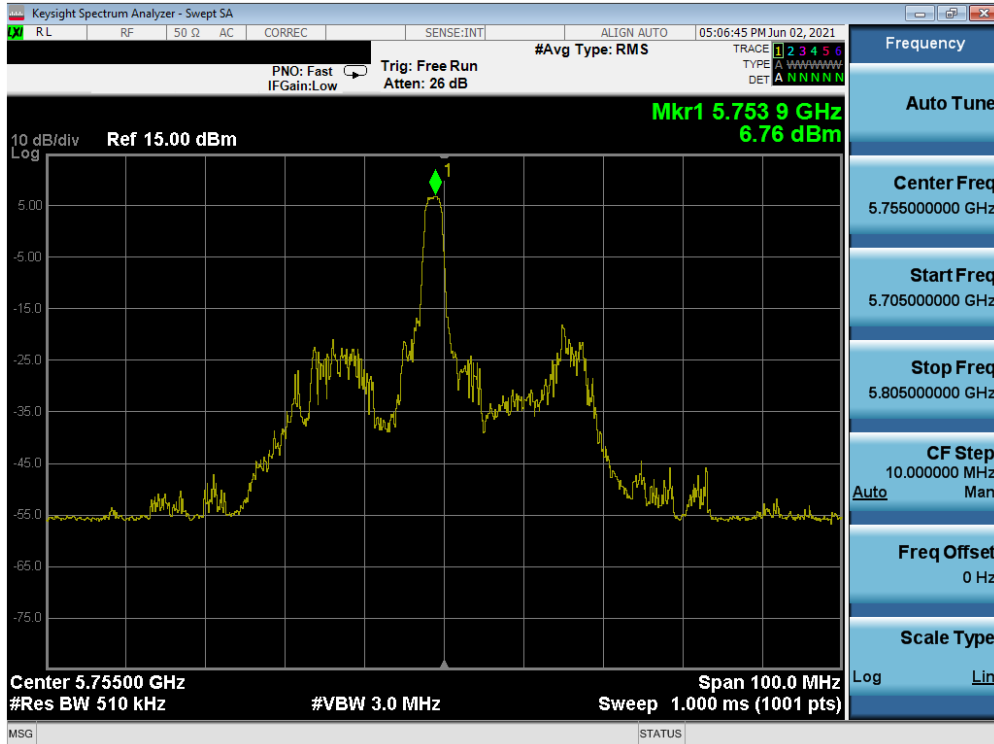
Plot 7-214. Power Spectral Density Plot MIMO ANT2 (40MHz BW 802.11ax – 26 Tones (UNII Band 3) – Ch. 151)
