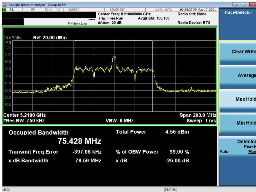
Plot 7-48. 26dB Bandwidth Plot MIMO (80MHz BW 802.11ax – 26 Tones (UNII Band 1) – Ch. 42)
