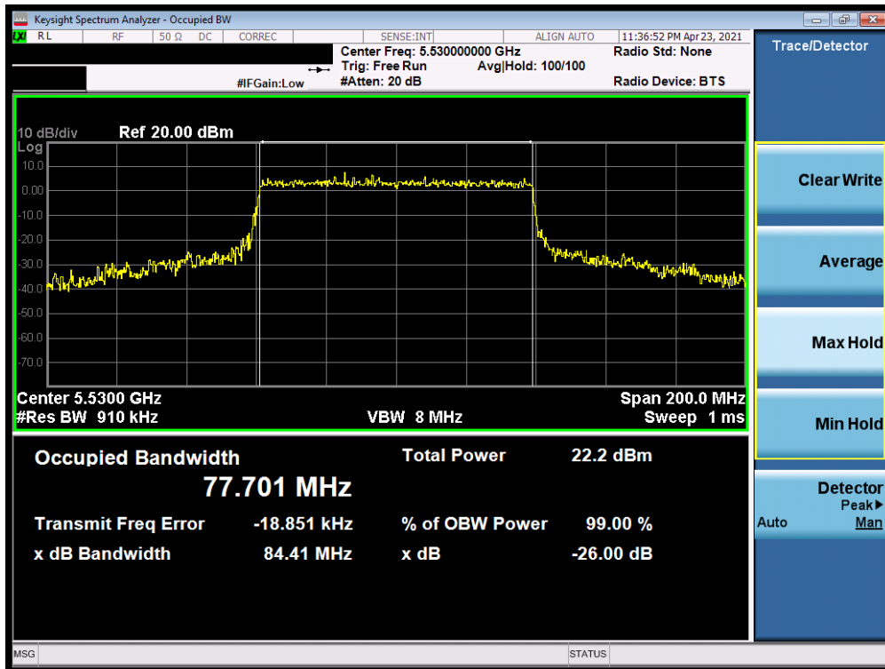
Plot 7-40. 26dB Bandwidth Plot SISO ANT1 (80MHz BW 802.11ax – 996 Tones (UNII Band 2C) – Ch. 106)
