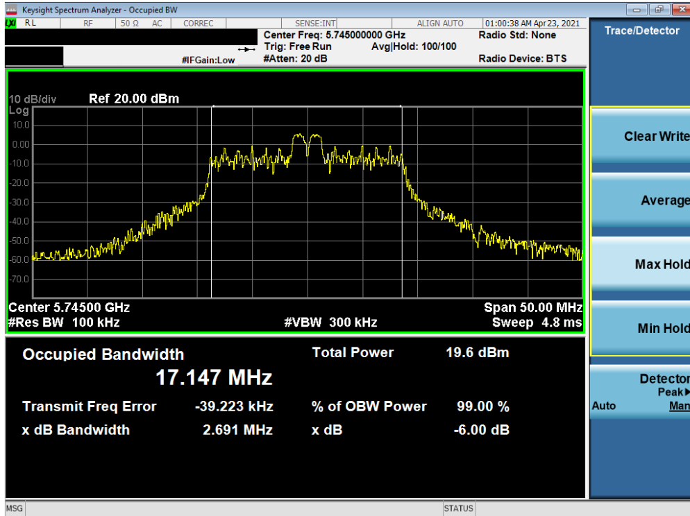
Plot 7-85. 6dB Bandwidth Plot SISO ANT1 (20MHz BW 802.11ax – 26 Tones (UNII Band 3) – Ch. 149)
