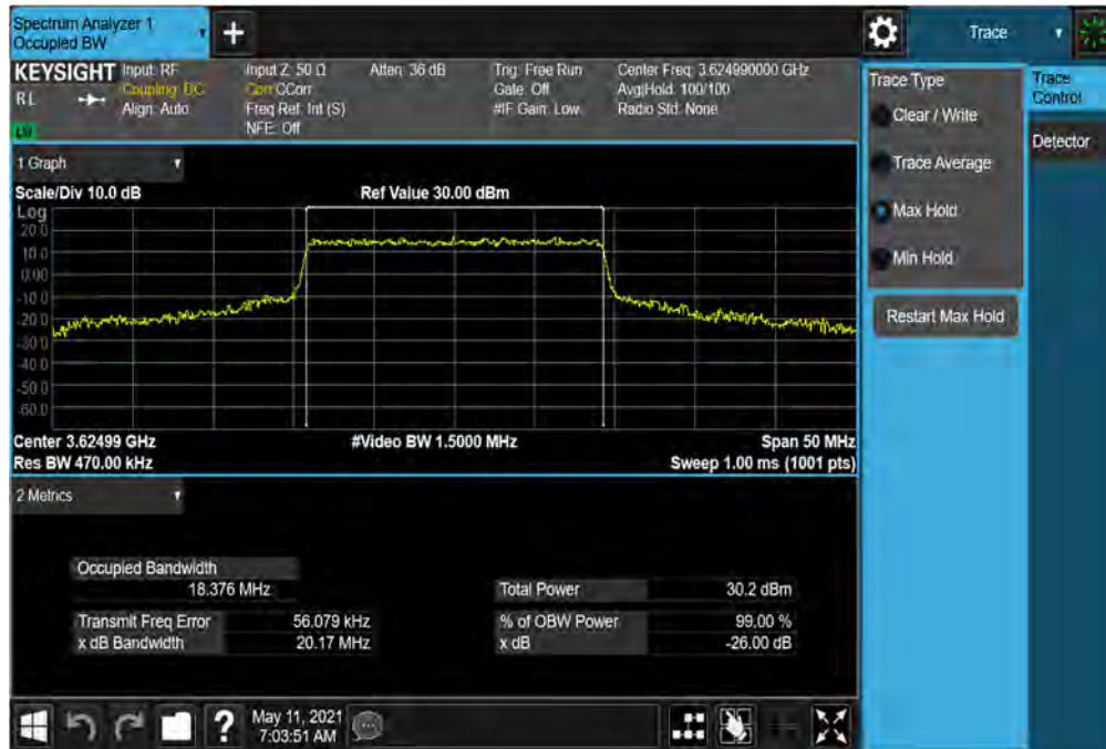
Plot 7-6. Occupied Bandwidth Plot (NR Band n48 - 20MHz CP-OFDM 16-QAM - Full RB Configuration)
