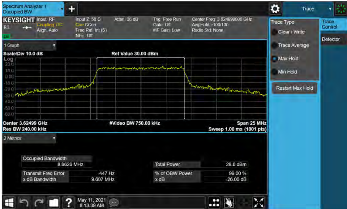
Plot 7-9. Occupied Bandwidth Plot (NR Band n48 - 10MHz CP-OFDM 16-QAM - Full RB Configuration)
