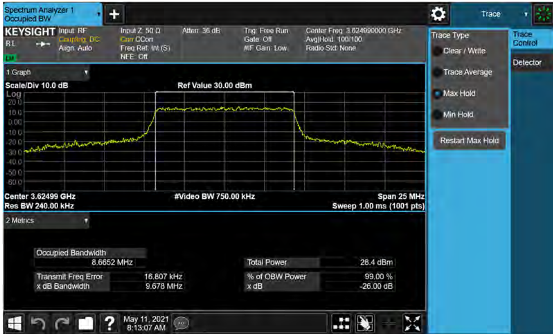
Plot 7-8. Occupied Bandwidth Plot (NR Band n48 - 10MHz CP-OFDM QPSK - Full RB Configuration)
