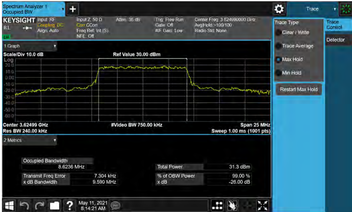
Plot 7-7. Occupied Bandwidth Plot (NR Band n48 - 10MHz DFT-s-OFDM \pi/2 -BPSK - Full RB Configuration)
