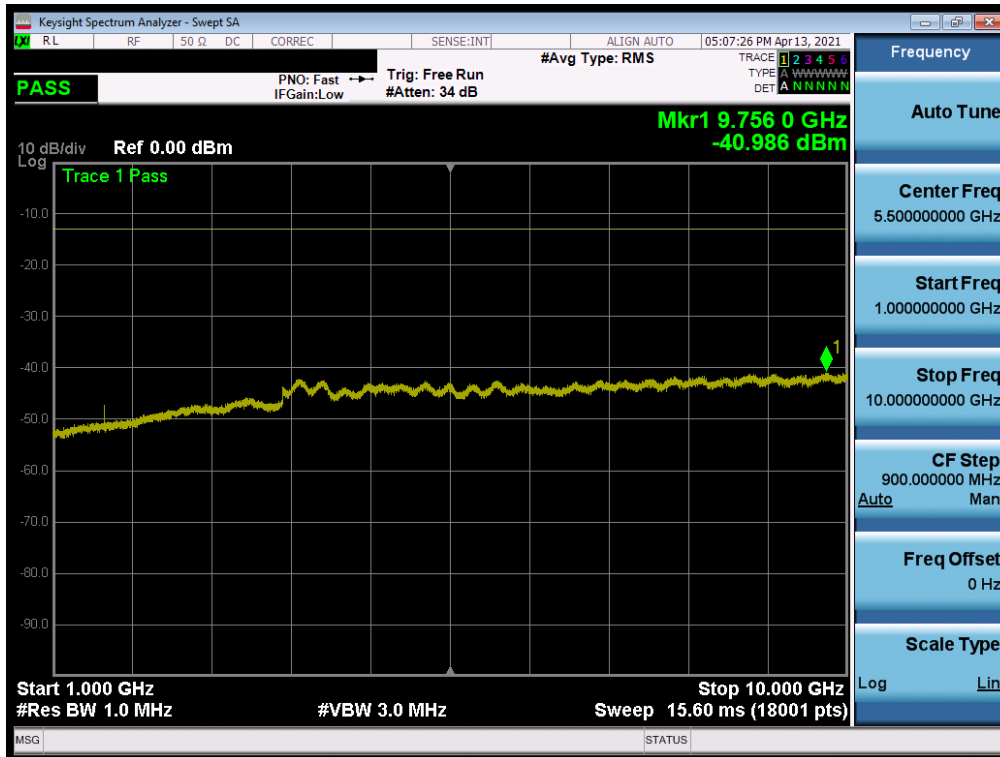
Plot 7-17. Conducted Spurious Plot (LTE Band 14 - 10MHz QPSK - RB Size 1, RB Offset 0)
