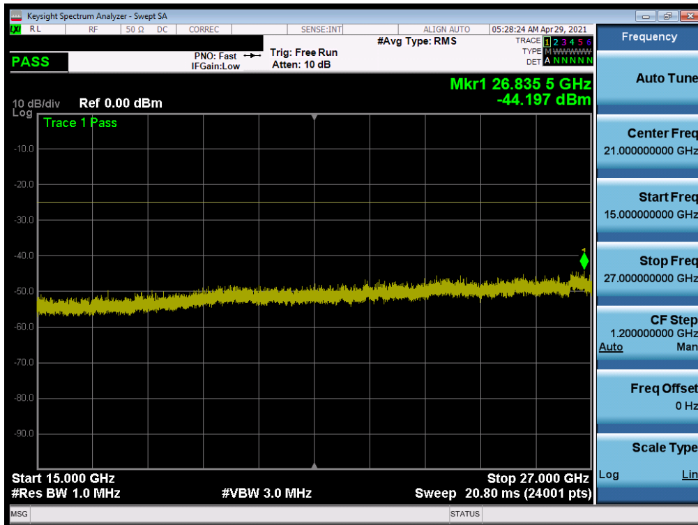
Plot 7-223. Conducted Spurious Plot (ULCA LTE B41(PC2) - 20MHz QPSK - RB Size 1, RB Offset 0 - High Channel)
