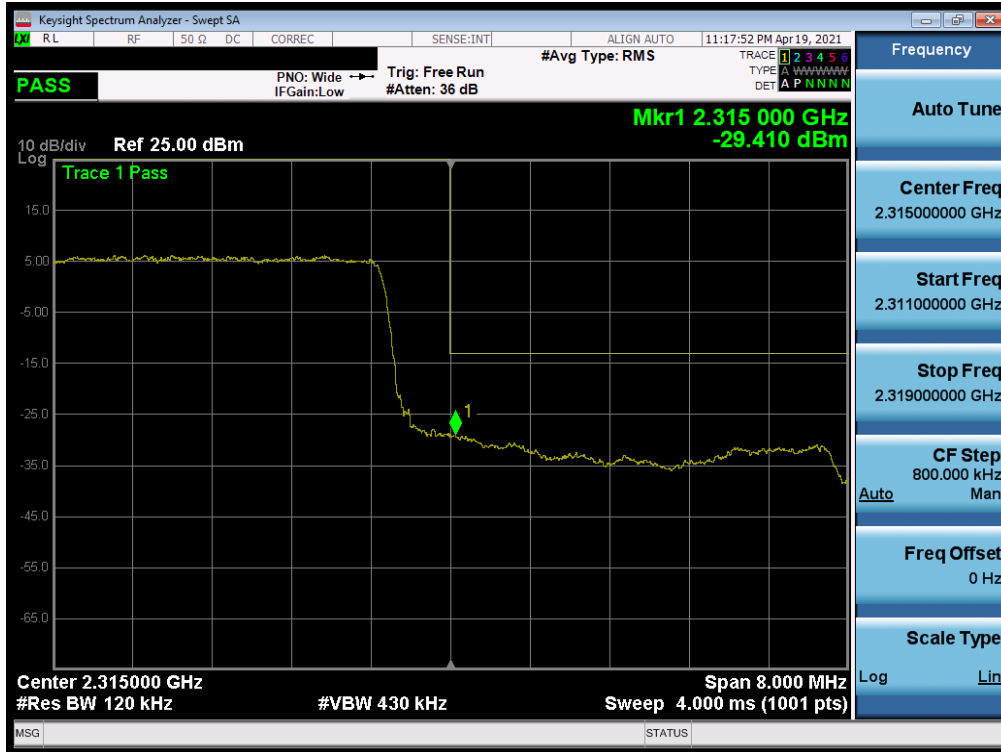
Plot 7-177. Upper Band Edge Plot (NR Band n30 - 10MHz CP-OFDM-QPSK – Full RB)
