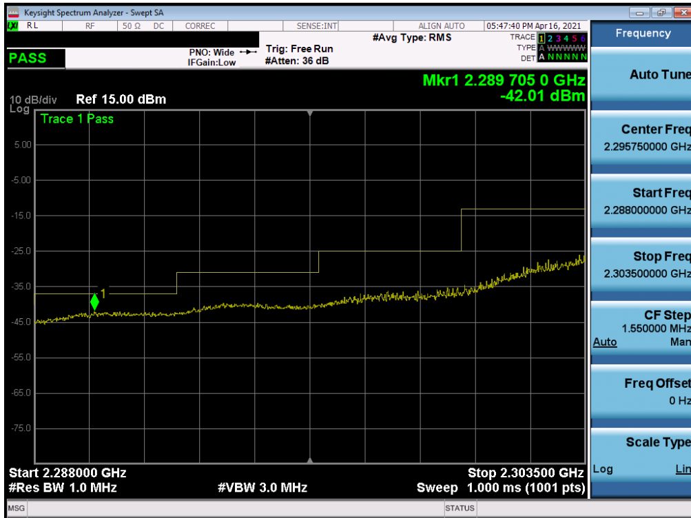
Plot 7-139. Extended Lower Band Edge Plot (LTE Band 30 - 5MHz QPSK – Full RB)
