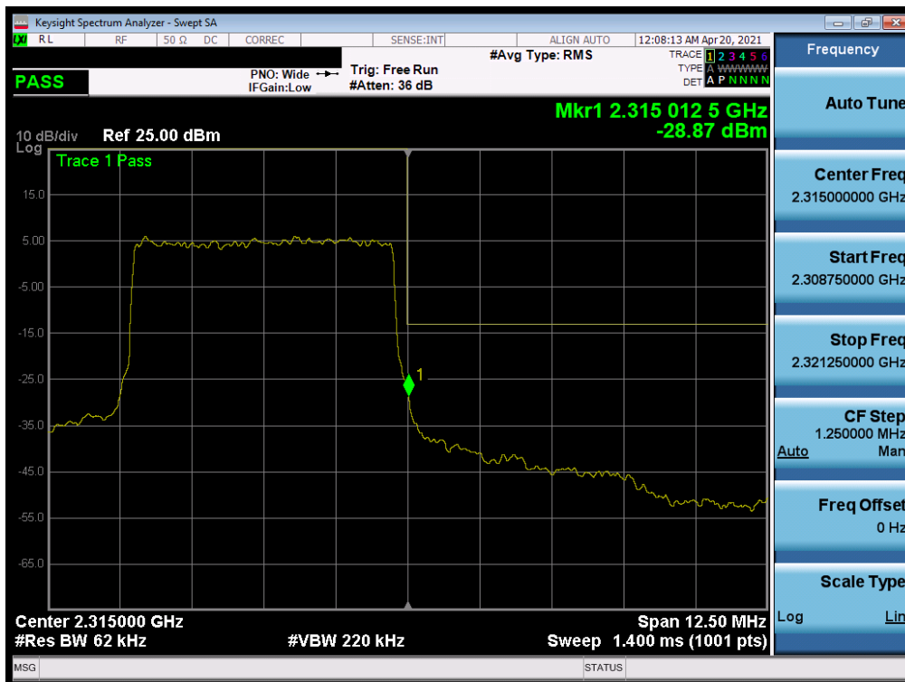
Plot 7-182. Upper Band Edge Plot (NR Band n30 - 5MHz CP-OFDM-QPSK – Full RB)
