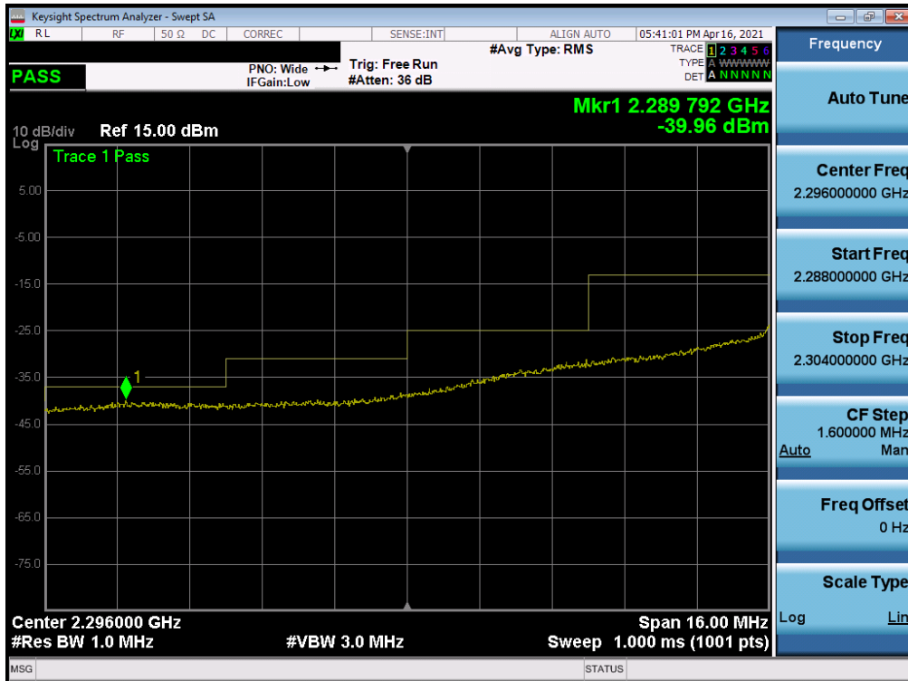
Plot 7-135. Extended Lower Band Edge Plot (LTE Band 30 - 10MHz QPSK – Full RB)
