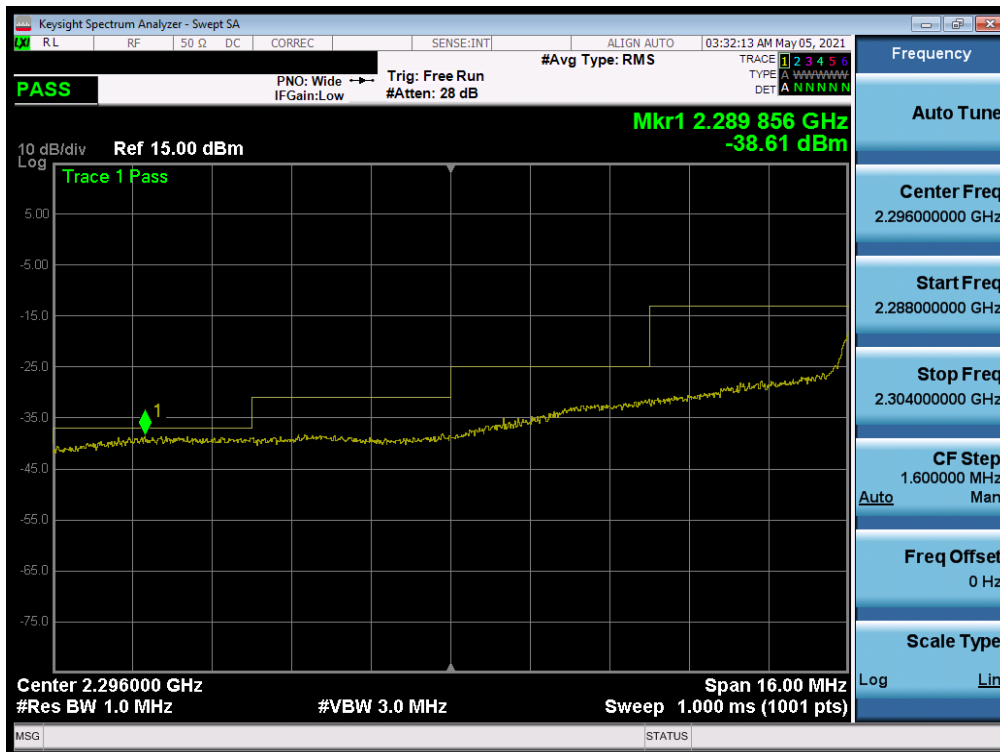
Plot 7-176. Extended Lower Band Edge Plot (NR Band n30 - 10MHz CP-OFDM-QPSK – Full RB)
